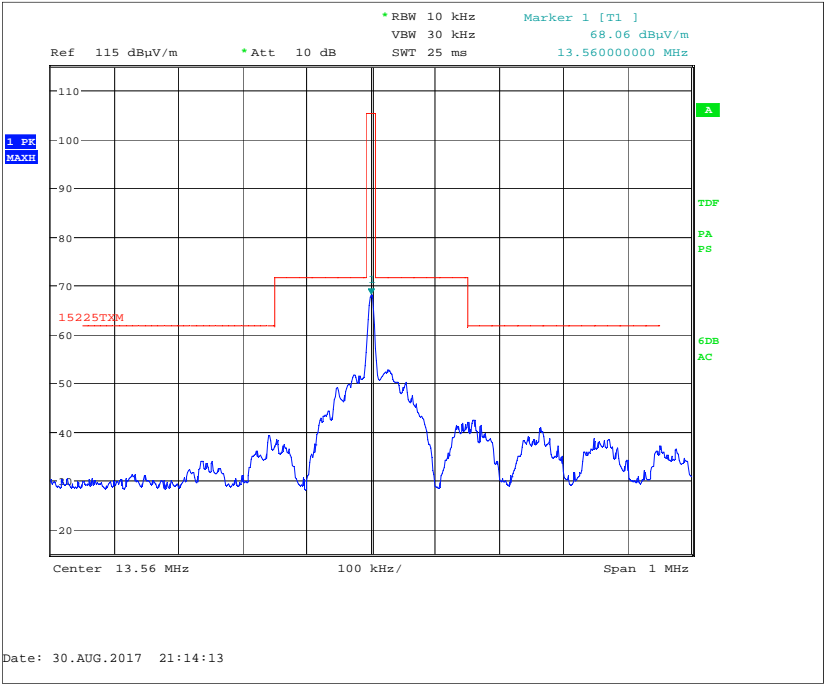
Figure 2 – Plot of the Fundamental (13.56 MHz)
