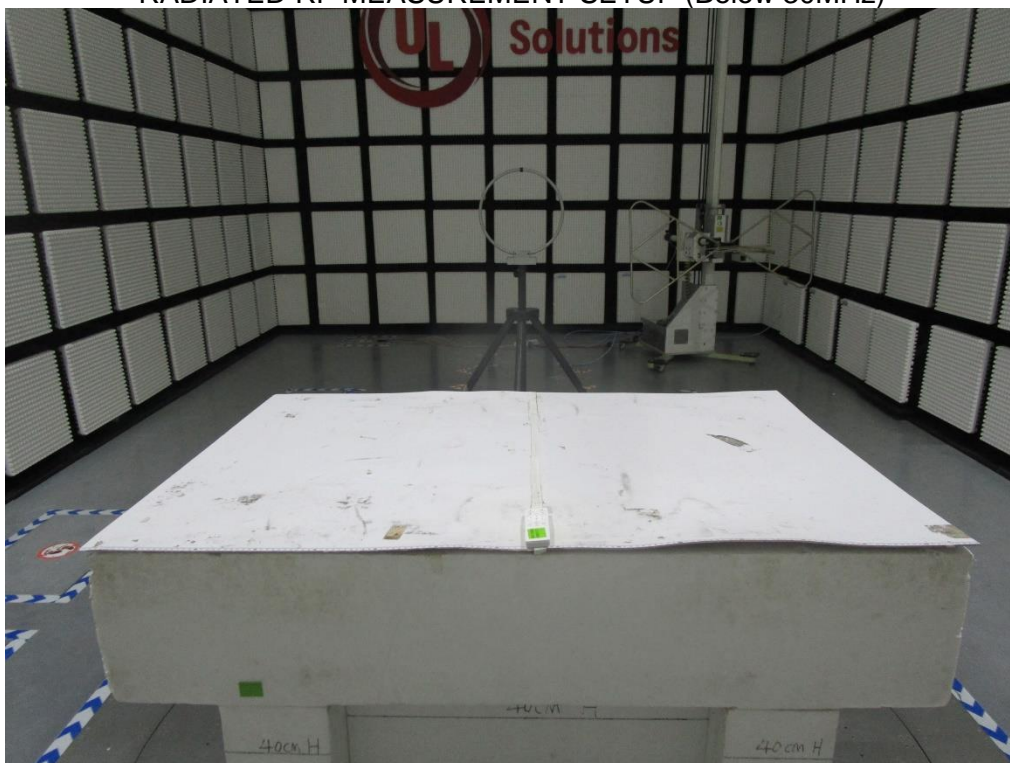
RADIATED RF MEASUREMENT SETUP (Below 30MHz)
