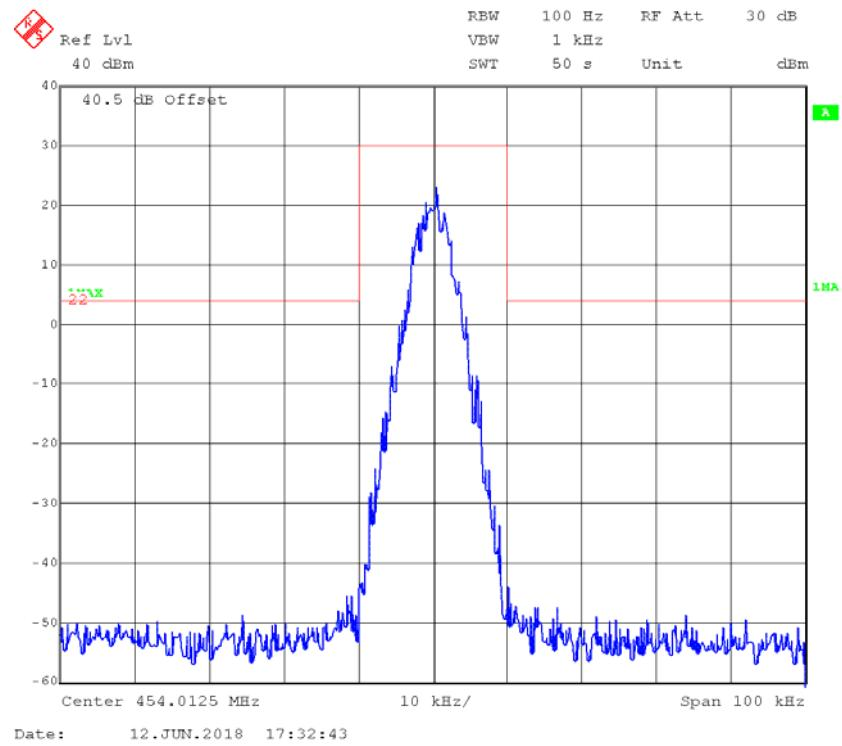
**FCC §2.1051 & §22.861 & §74.462 & § 80.211 & §90.210 - SPURIOUS EMISSIONS AT ANTENNA TERMINALS****Applicable Standard**
