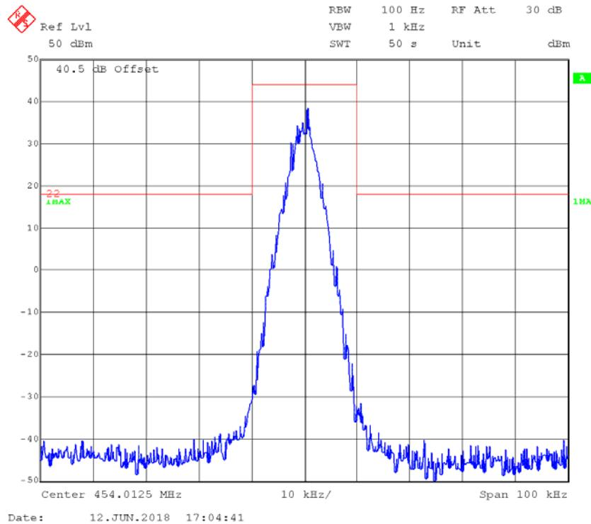
**4FSK,12.5kHz,Low Power - Frequency 454.0125 MHz: 99% Occupied & 26 dB Bandwidth**
