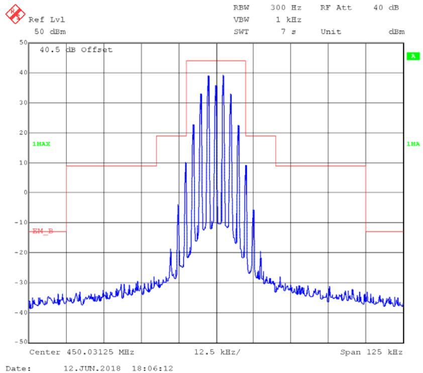
**FM,25kHz,Low Power - Frequency 450.03125 MHz: 99% Occupied & 26 dB Bandwidth**
