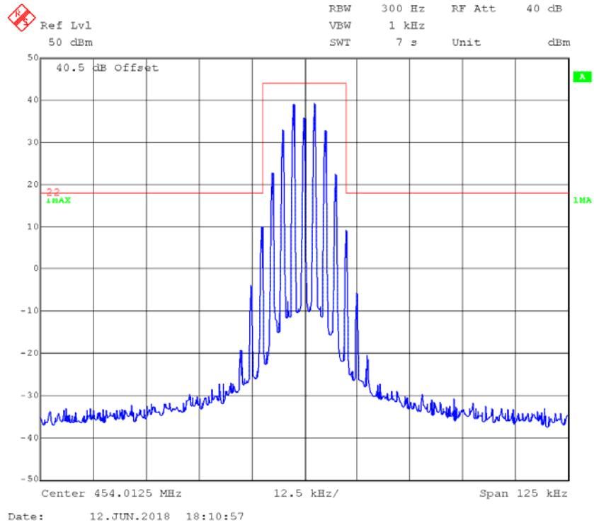
**FM,25kHz,Low Power - Frequency 454.0125 MHz: 99% Occupied & 26 dB Bandwidth**
