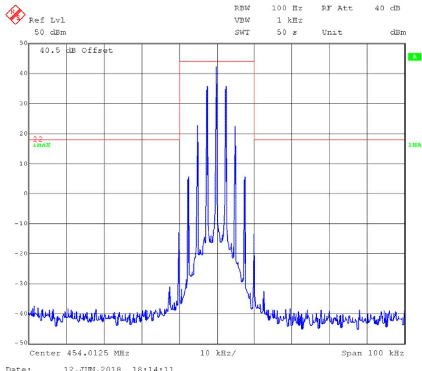
**FM,12.5kHz,Low Power - Frequency 454.0125 MHz: 99% Occupied & 26 dB Bandwidth**
