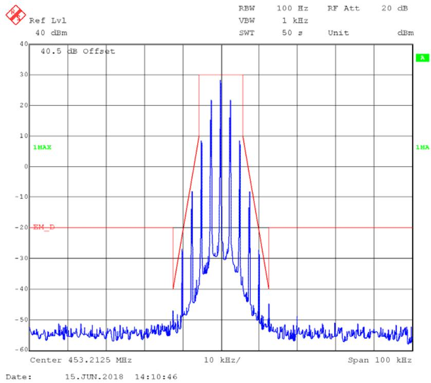
**4FSK,12.5kHz,High Power - Frequency 453.2125 MHz: 99% Occupied & 26 dB Bandwidth**
