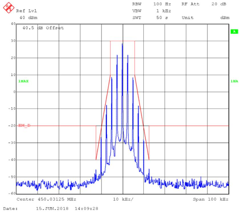
**FM,25kHz,High Power - Frequency 450.03125 MHz: 99% Occupied & 26 dB Bandwidth**
