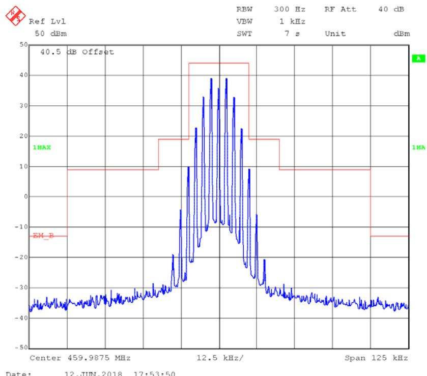
**FM,25kHz,Low Power - Frequency 459.9875 MHz: 99% Occupied & 26 dB Bandwidth**
