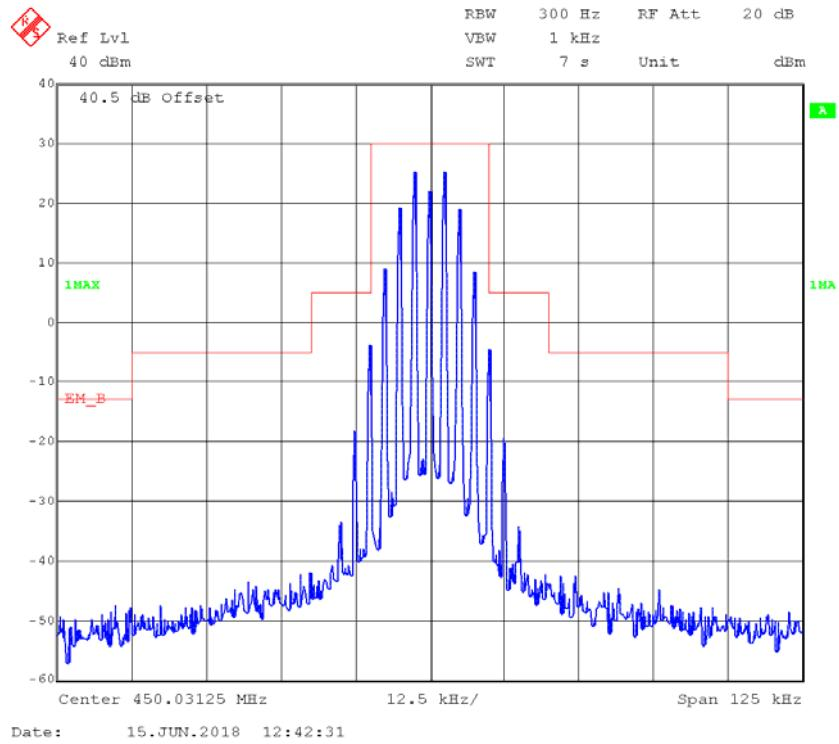
**4FSK,12.5kHz,High Power - Frequency 450.03125 MHz: 99% Occupied & 26 dB Bandwidth**
