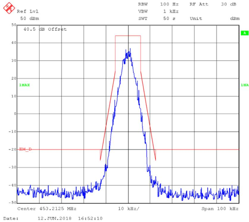
**4FSK,12.5kHz,Low Power - Frequency 453.2125 MHz: 99% Occupied & 26 dB Bandwidth**
