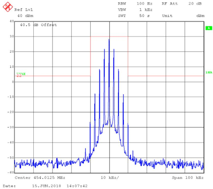
**FM,25kHz,High Power - Frequency 454.0125 MHz: 99% Occupied & 26 dB Bandwidth**
