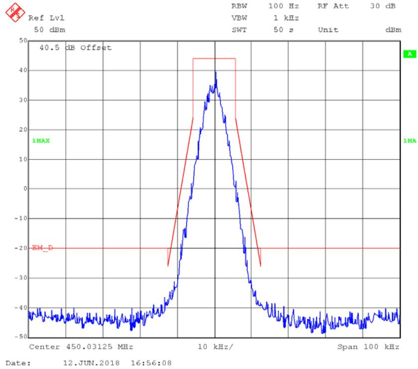
**4FSK,12.5kHz,Low Power - Frequency 450.03125 MHz: 99% Occupied & 26 dB Bandwidth**
