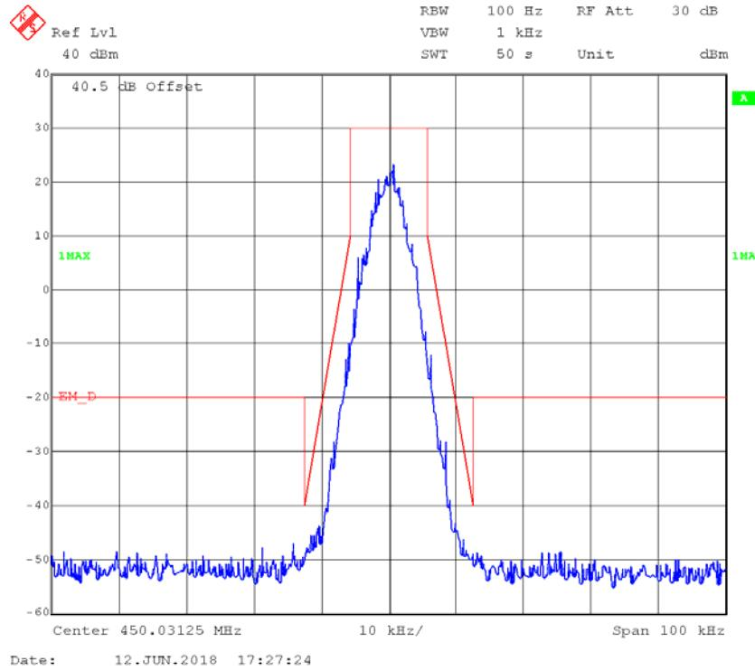
**Part 22****FM,12.5kHz,High Power - Frequency 454.0125 MHz: 99% Occupied & 26 dB Bandwidth**
