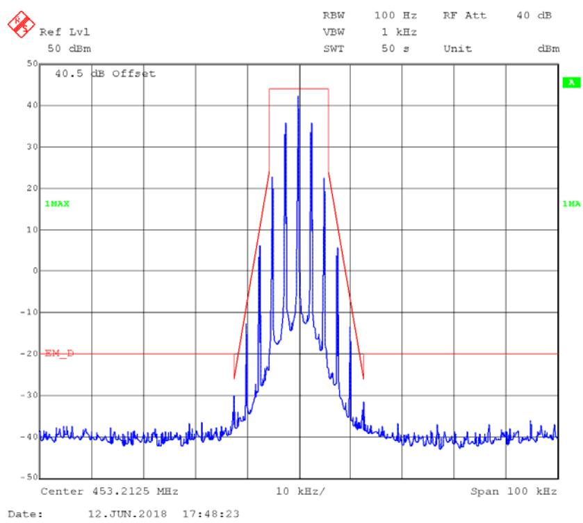
**FM,12.5kHz,Low Power - Frequency 453.2125 MHz: 99% Occupied & 26 dB Bandwidth**
