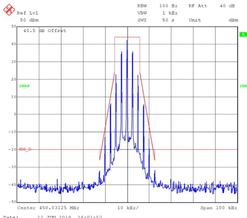
**FM,12.5kHz,Low Power - Frequency 450.03125 MHz: 99% Occupied & 26 dB Bandwidth**
