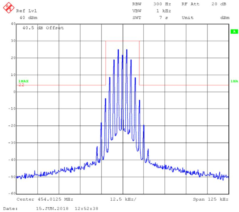
**4FSK,12.5kHz,High Power - Frequency 454.0125 MHz: 99% Occupied & 26 dB Bandwidth**
