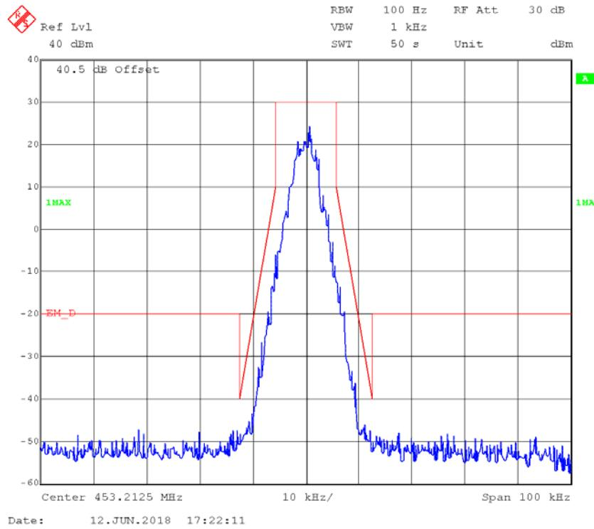
**Part 80:****FM,25kHz, High Power - Frequency 459.9875 MHz: 99% Occupied & 26 dB Bandwidth**
