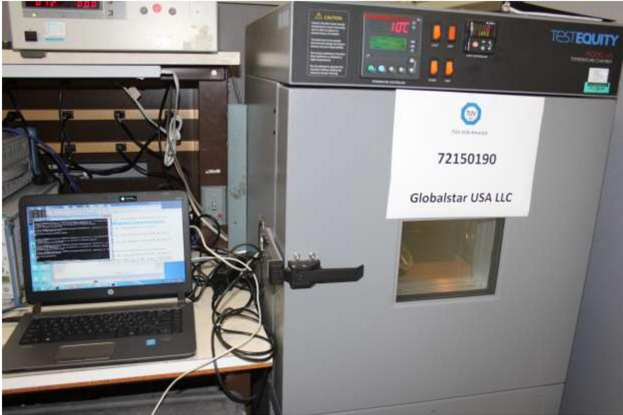
**Frequency Stability/Voltage Variation Test Setup**
