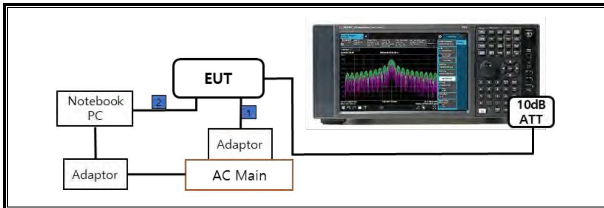
**SETUP DIAGRAM FOR TESTS (RADIATED TEST SETUP)**
