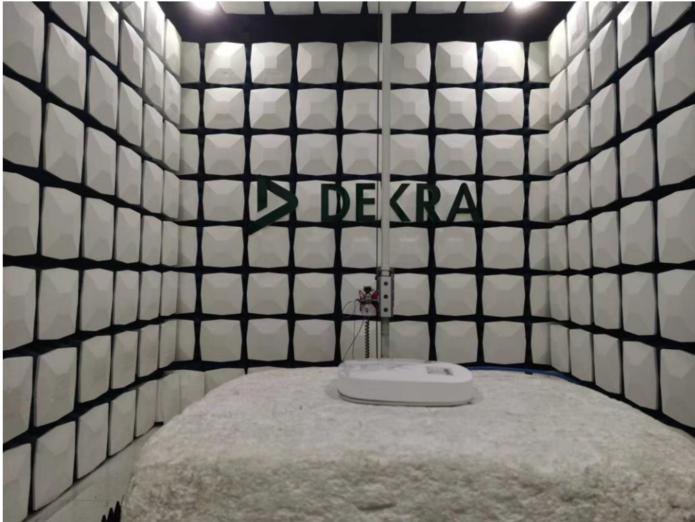
Description: Radiated Emission Test Setup for 1~18GHz
