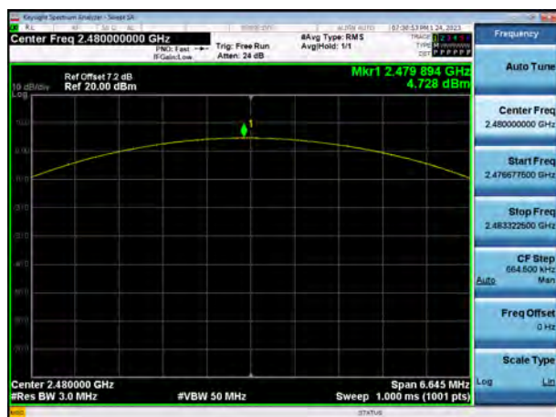
Ant. 1 8DPSK : Peak Power (CH.78)
