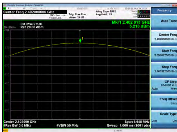
Ant. 1 8DPSK : Peak Power (CH.39)
