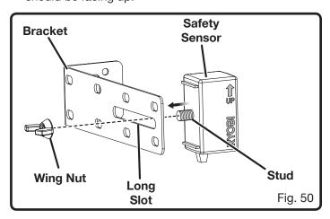
**NOTE:** The top of the sensor should be between four and six inches above the floor.
