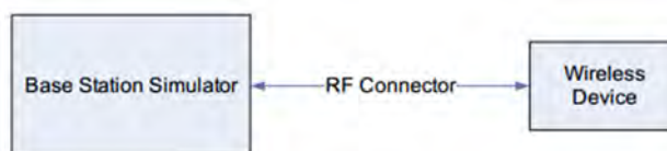
Figure 9.1 Power Measurement Setup
