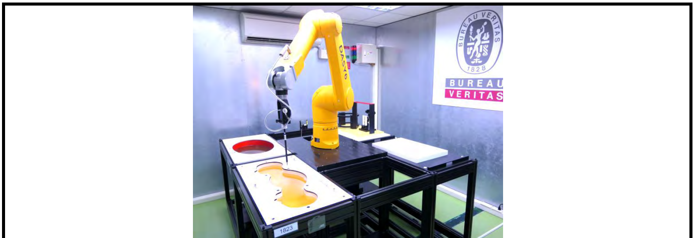
Fig-3.2 SPEAG DASY6 System
