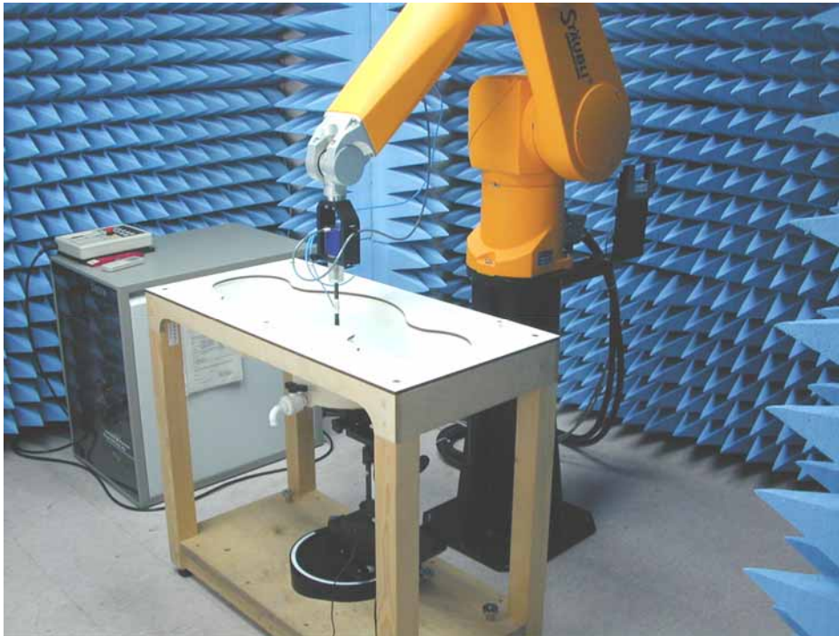
Fig.1 Photograph of the SAR measurement System
