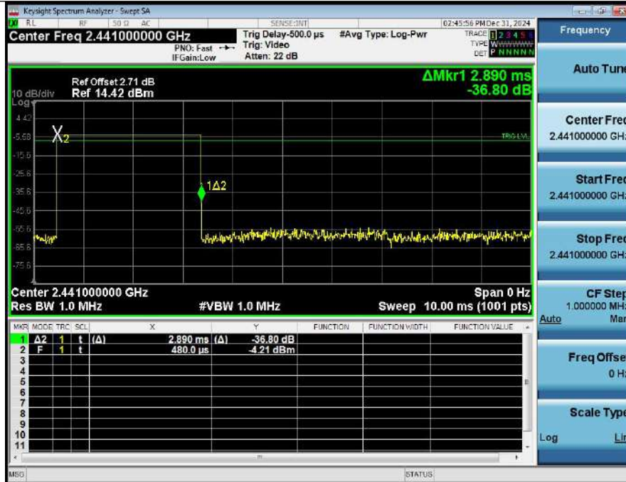
Dwell Time (Hopping) NVNT_ANT1_1-DH5_2441_00_Accumulated
