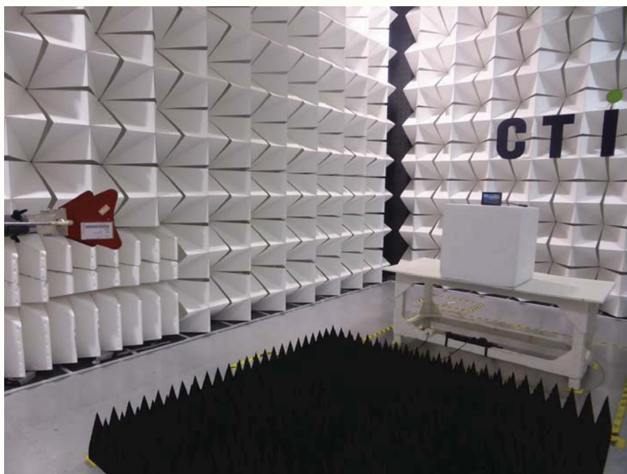
Radiated spurious emission Test Setup-2(Above 1GHz)
