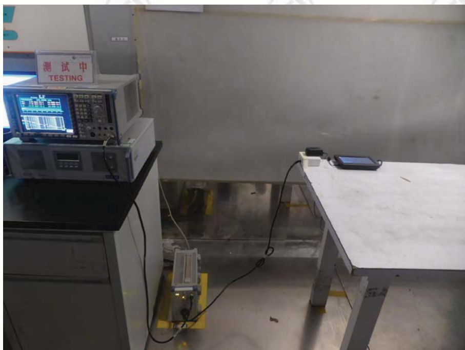
Conducted emission Test Setup
