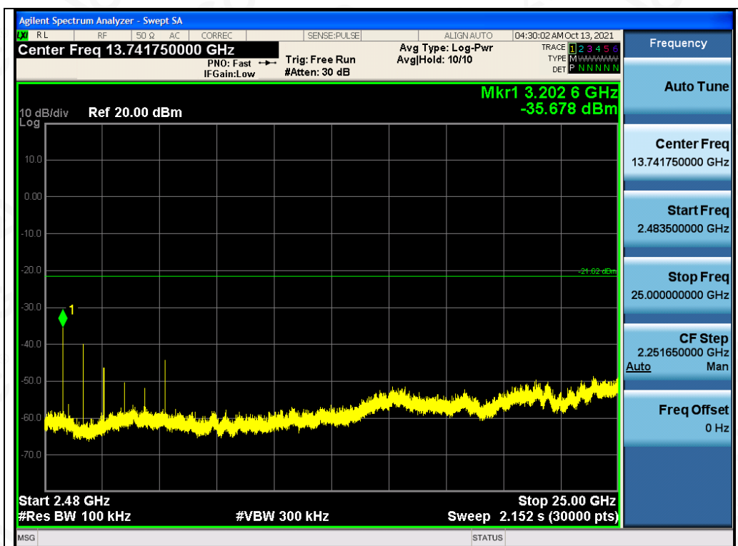
Test_Graph_EDR_ANT1_2402_3Mbps_Higher Band Emissions
