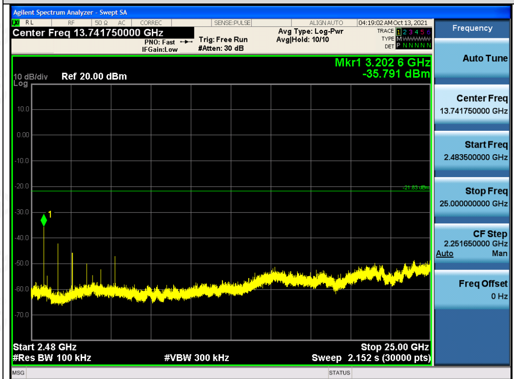
Test_Graph_EDR_ANT1_2402_2Mbps_Higher Band Emissions
