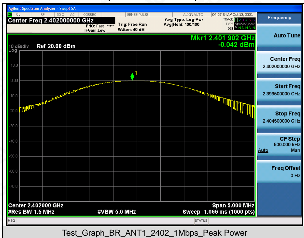
Test Graphs of Conducted Output Power
