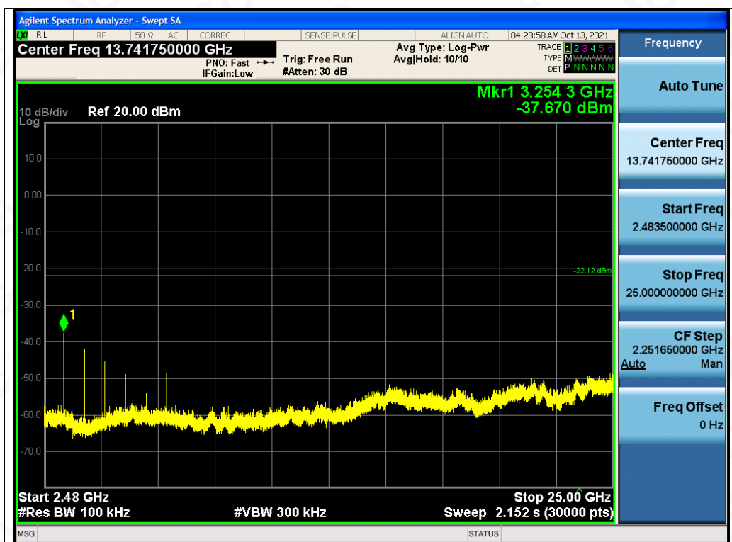
Test_Graph_EDR_ANT1_2441_2Mbps_Higher Band Emissions
