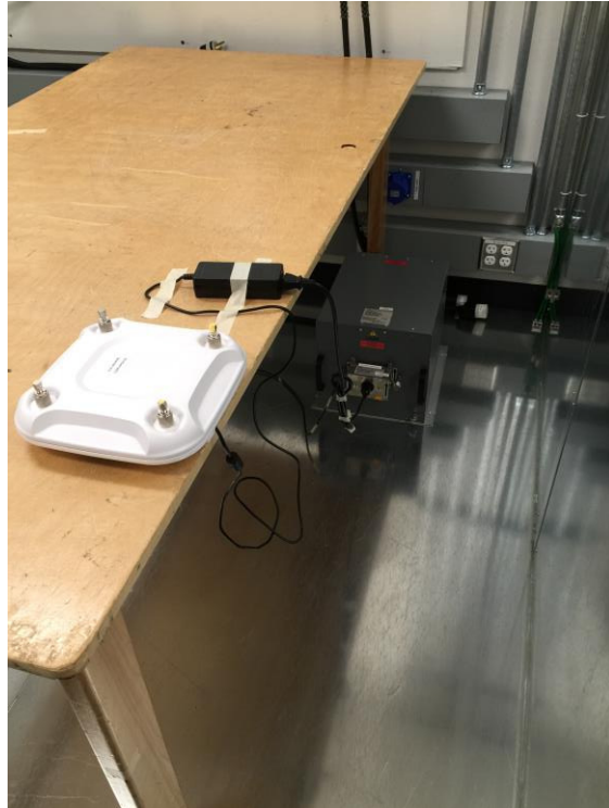
AIR-CAP3702P-B-K9 AC Conducted Emissions setup photo
