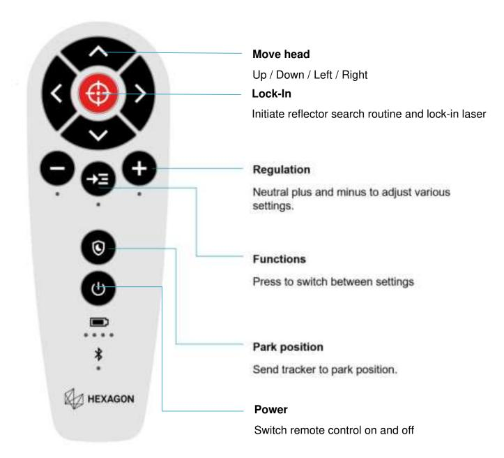
Piicture: Remote control of LASERTRACER and its basic functions
