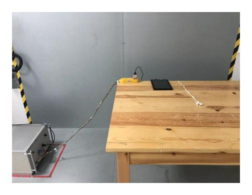
Set-up for Radiated Emission (RE), Below 1GHz
