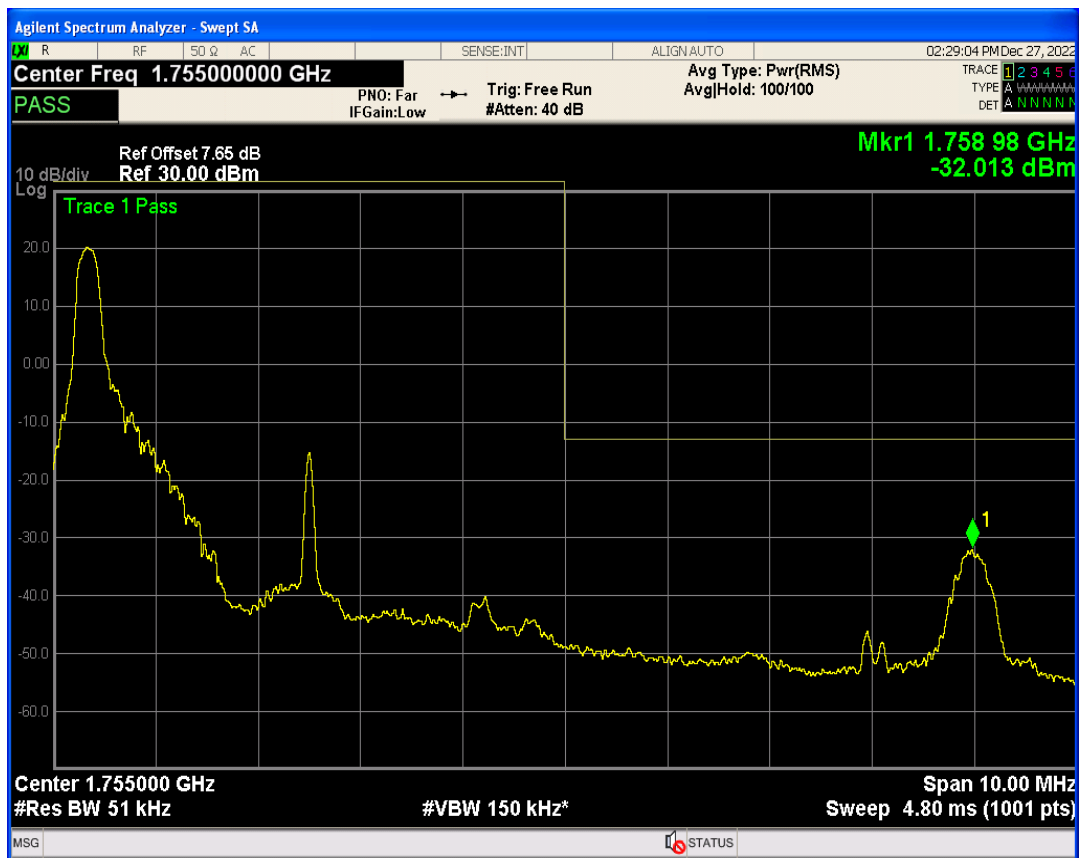
Band4 QAM16 BW=5MHz Channel=19975 RB Size=25 Position=#0
