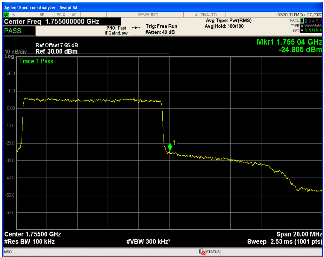
Band4 QAM16 BW=10MHz Channel=20350 RB Size=1 Position=#Max
