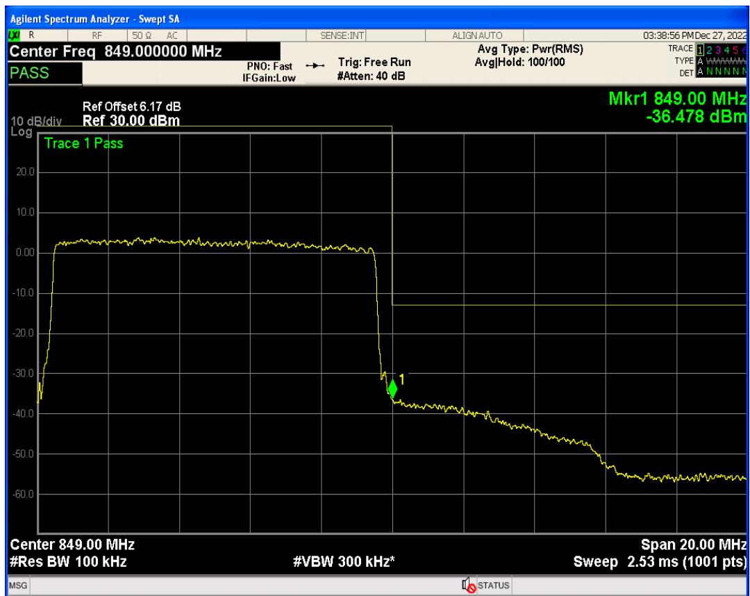
Band7 QPSK BW=5MHz Channel=20775 RB Size=1 Position=#0
