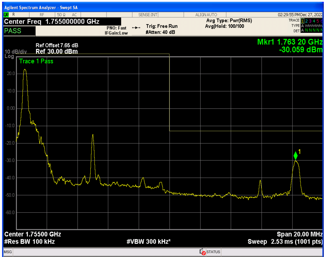
Band4 QPSK BW=10MHz Channel=20350 RB Size=1 Position=#Max
