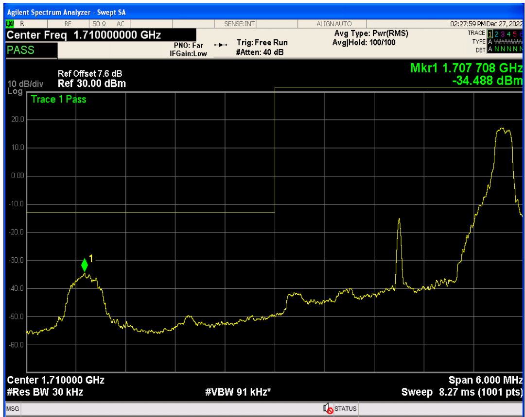
Band4 QAM16 BW=3MHz Channel=19965 RB Size=15 Position=#0
