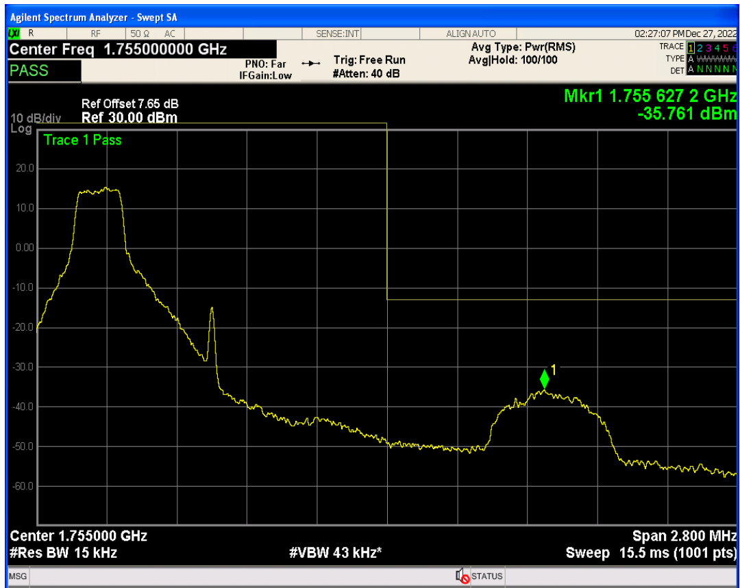
Band4 QPSK BW=1.4MHz Channel=20393 RB Size=1 Position=#Max
