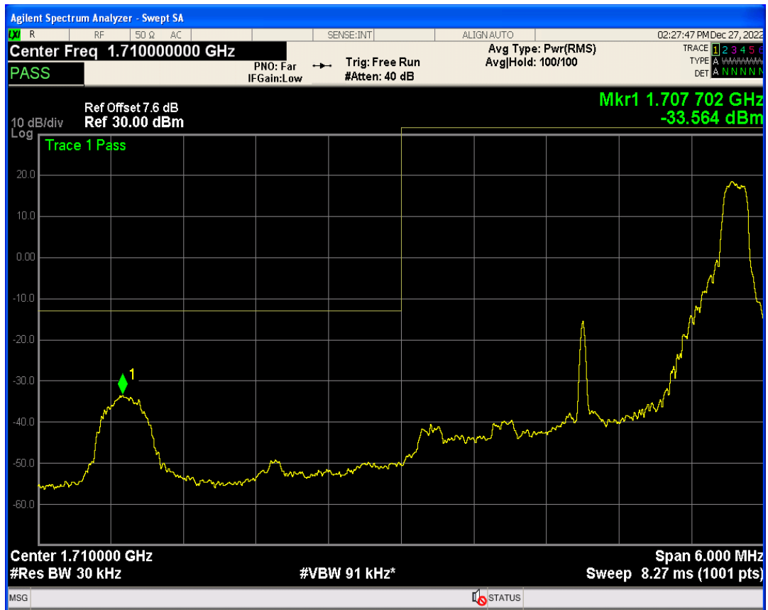
Band4 QPSK BW=3MHz Channel=19965 RB Size=1 Position=#0
