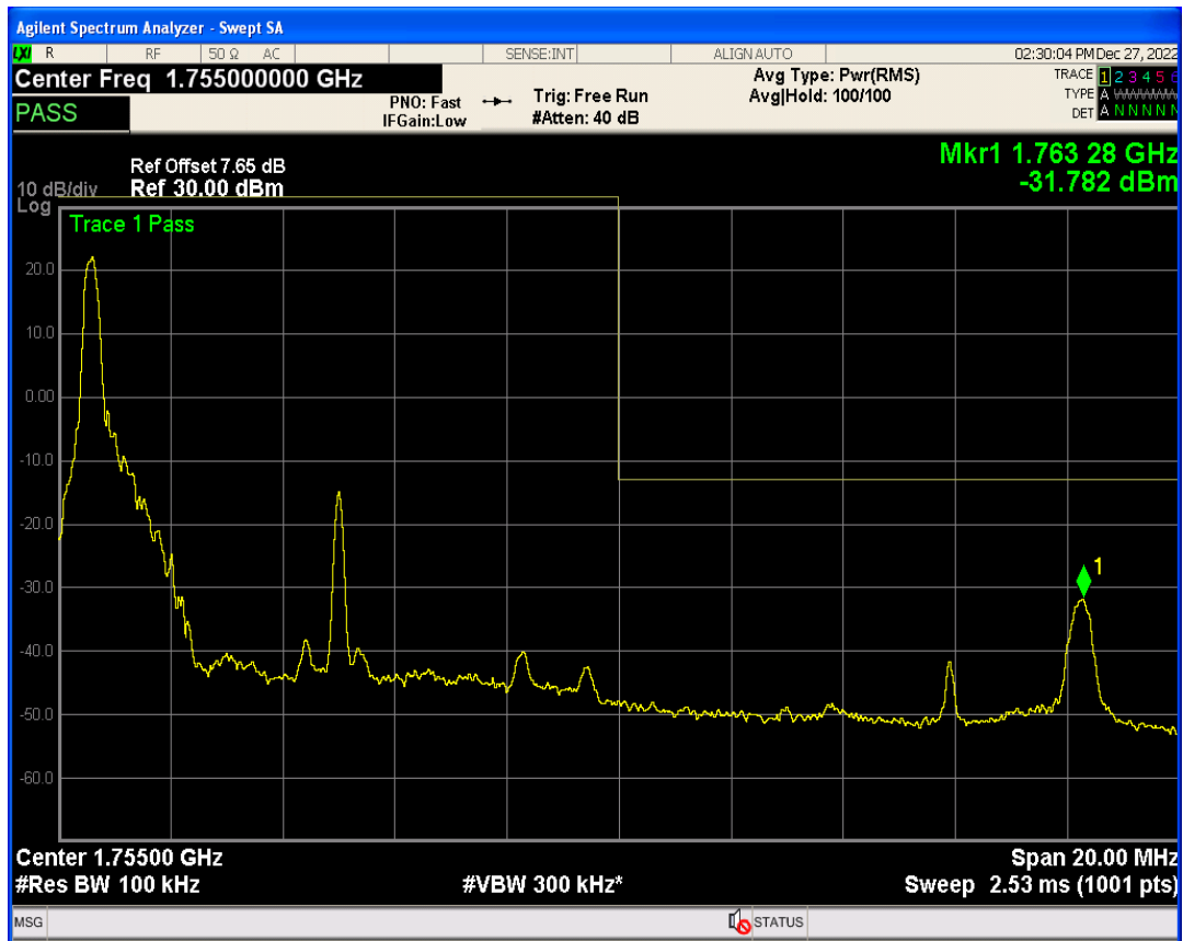
Band4 QAM16 BW=10MHz Channel=20350 RB Size=50 Position=#0
