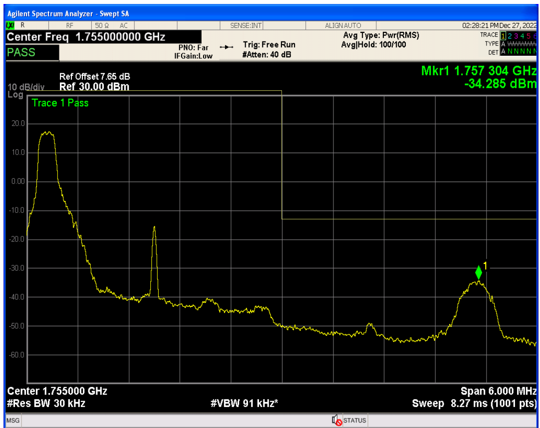
Band4 QAM16 BW=3MHz Channel=20385 RB Size=1 Position=#Max
