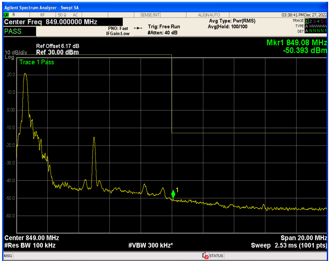
Band5 QPSK BW=10MHz Channel=20600 RB Size=1 Position=#Max
