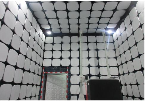
Remark: The transmitter part of the EUT was kept on the high 1.5m above 1GHz according to the lifting platform during the test.
