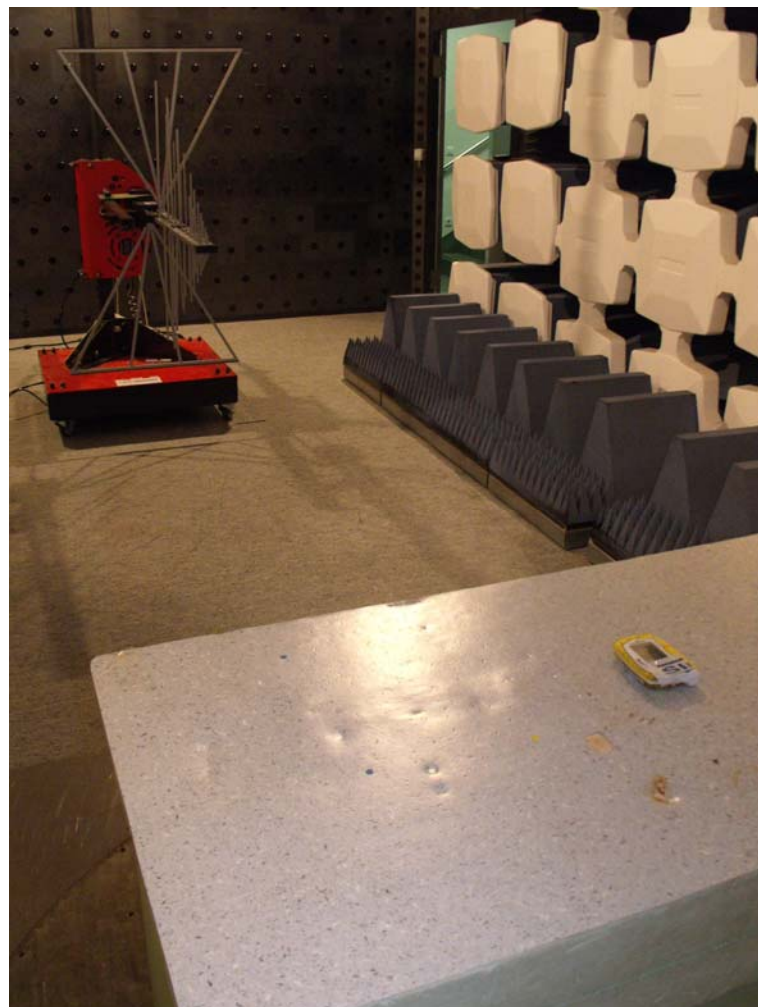
Figure 2: Radiated emission test – over 30 MHz
