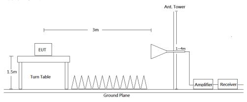
Radiated emission tests were performed in the 3 meters chamber test site, using the setup accordance with the ANSI C63.10-2013. The specification used was the FCC Part 15.209, FCC 15.407, RSS-247, RSS-GEN Limits.
