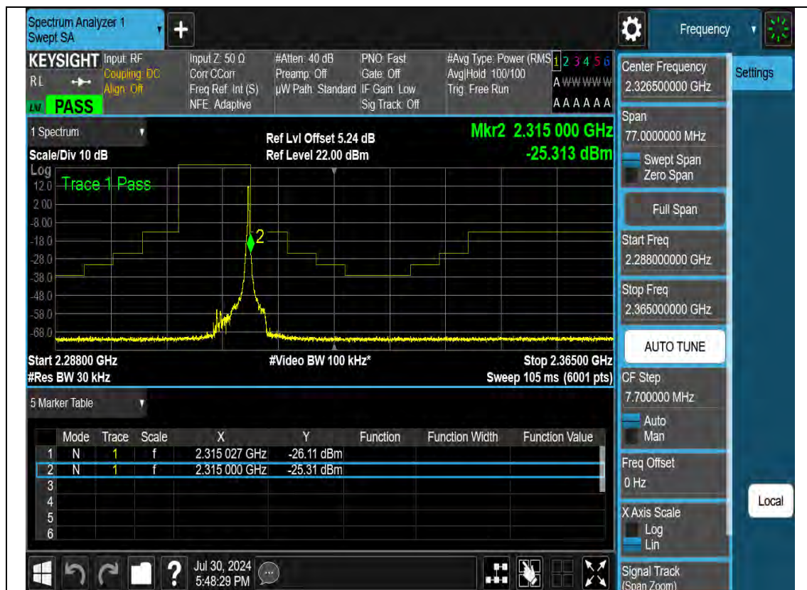
N30-10M-Bandedge-M-DFT-s-OFDM-Pi2 BPSK-Outer Full
