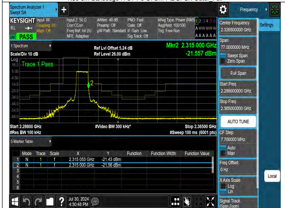
N30-5M-Bandedge-H-DFT-s-OFDM-Pi2 BPSK-1RB MAX
