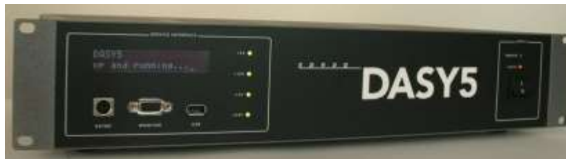
Fig. 8.5 Photo of Server for DASY5
