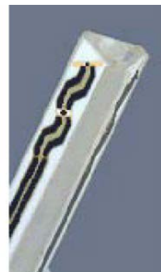
Figure 2.3 Probe Thick-Film Technique
