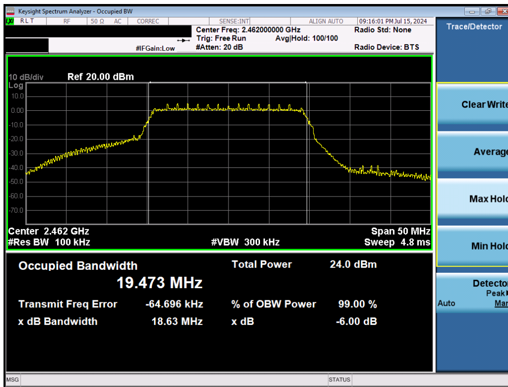
Plot 7-9. 6dB Bandwidth & 99% OBW Plot (802.11n (2.4GHz) – Ch. 11) – MCS0
