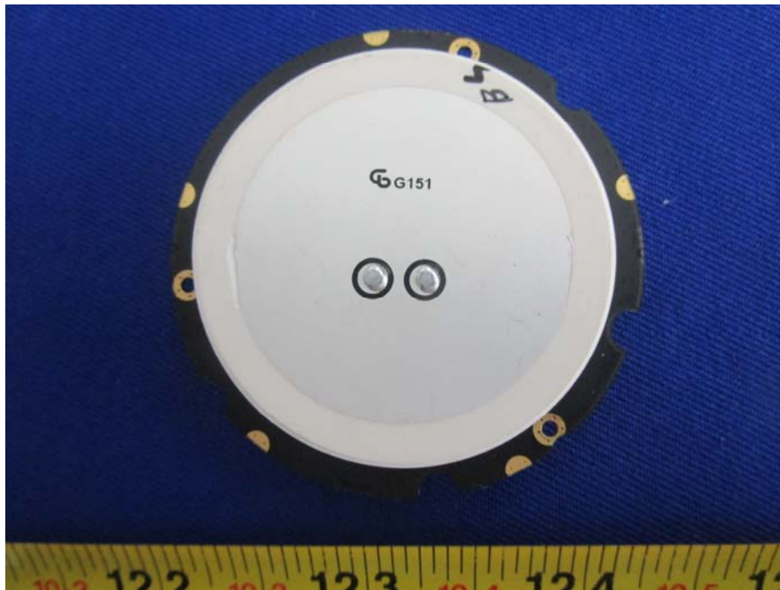
EUT – GPS Module Top & Antenna View
