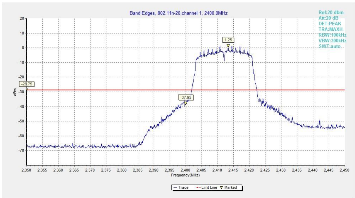
Fig.23 Band Edges (802.11n-HT20, CH 1)
