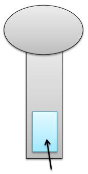
Label is affixed in the battery compartment. Batteries are not pre-installed during marketing. Users will see the label as they install the batteries to operate this device.
