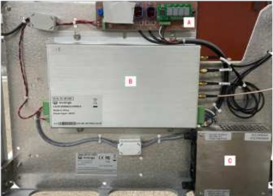
Figure 7.1: Latest LSP3A-LR Clear PEM and Power Supply Unit Location Bottom right
