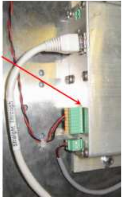
Figure 5.16: Peripherals & GPIO Green Connector Pin Out & Location
