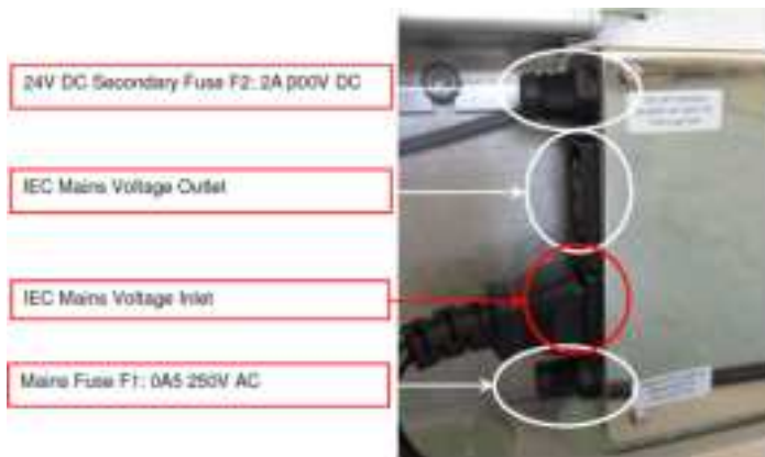
Figure 7.2: Mains Fuses Location and Ratings
