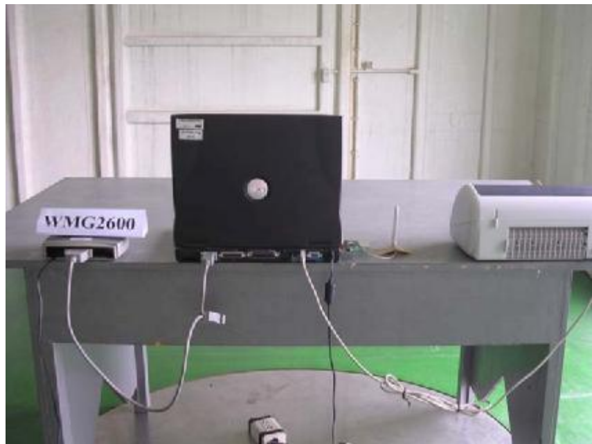
Photo 2: Radiated Emission Test Set-up
