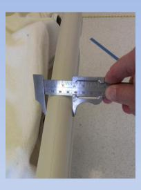
For widths from ½" to 1-1/4" (12mm to 31mm) use part number **5835-500**
