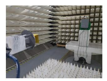
Photograph No.6 Frequency stability measurement setup
