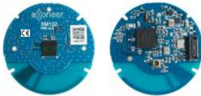
Figure 1. XM122 connectivity module Top view (left) and XM122 bottom view (right).
