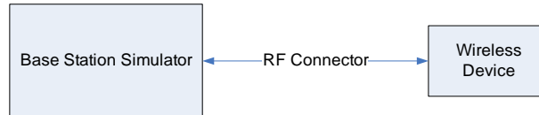
Figure 9-3 Power Measurement Setup
