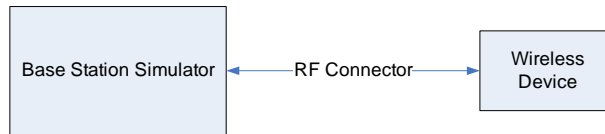
Figure 9-2 Power Measurement Setup
