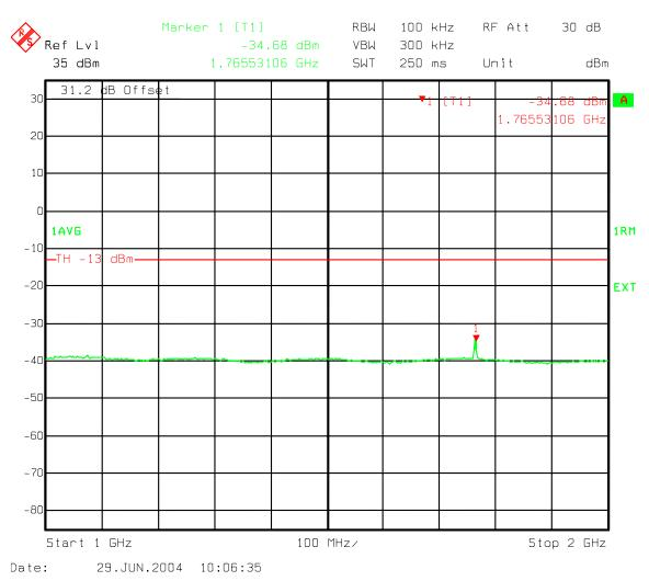
Figure 129: Combination Three Carriers 2-IS856 16QAM, 1-IS95 - B Band Spurious emissions 1000-2000 MHz
