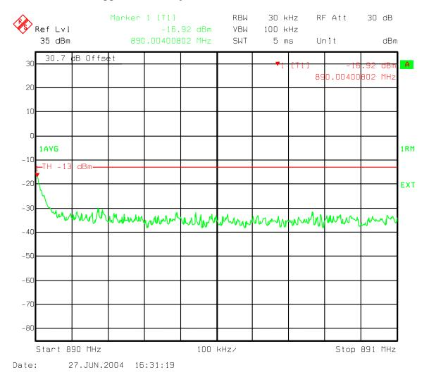
Figure 163: Three Carriers IS856 QPSK - Ch 560, 601, 642 Upper B Band adjacent 1 MHz band emissions 890-891 MHz
