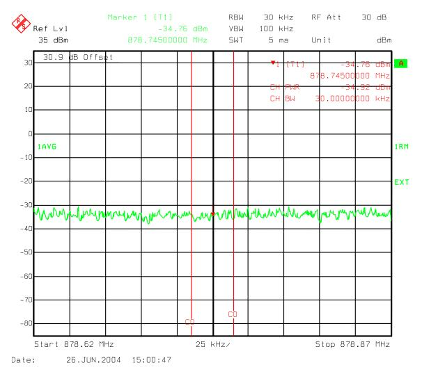
Figure 101: Three Carriers IS856 16QAM - Industry Canada 1.98 MHz offset Lower 30 kHz Chan Power Ch 358, 399, 440
