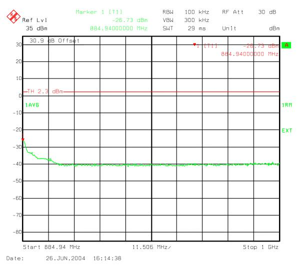
Figure 149: Three Carriers IS856 8PSK - B Band Spurious emissions Upper 1 MHz Band Edge to 1 GHz
