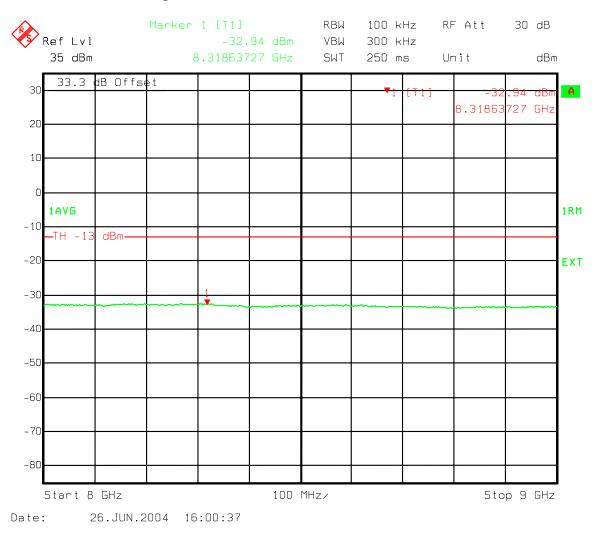
Figure 158: Three Carriers IS856 8PSK - B Band Spurious emissions 8000-9000 MHz
