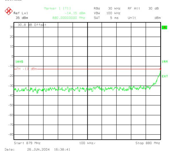
Figure 161: Three Carriers IS856 QPSK - B Band Ch 358, 399, 440 IS856 Adjacent 1MHz Lower emissions 879-880MHz
