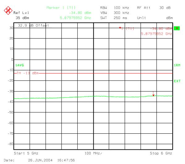
Figure 177: Three Carriers IS856 QPSK - B Band Spurious emissions 5000-6000 MHz
