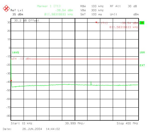
Figure 103: Three Carriers IS856 16QAM - B Band Spurious emissions 10kHz-400 MHz
