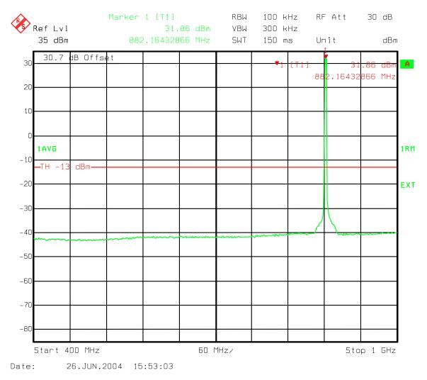
Figure 150: Three Carriers IS856 8PSK - B Band Spurious emissions 400-1000 MHz
