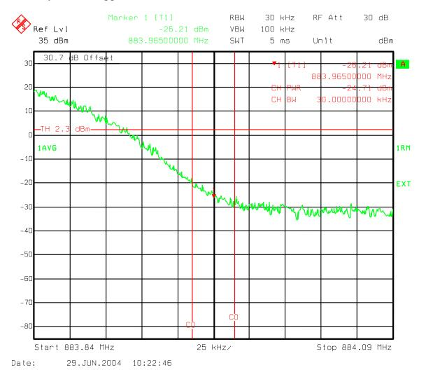
Figure 122: Combination Three Carriers 2-IS856 16QAM, 1-IS95 - Industry Canada Upper 750 kHz offset 30 kHz Chan Power Ch 358, 399, 440
