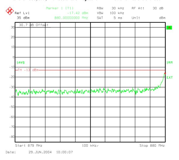
Figure 117: Combination Three Carriers 2-IS856 16QAM, 1-IS95 - B Band Ch 358, 399, 440 IS856 Adjacent 1MHz Lower emissions 879-880MHz
