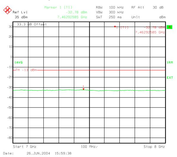
Figure 157: Three Carriers IS856 8PSK - B Band Spurious emissions 7000-8000 MHz
