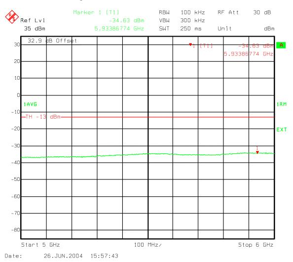
Figure 155: Three Carriers IIS856 8PSK - B Band Spurious emissions 5000-6000 MHz
