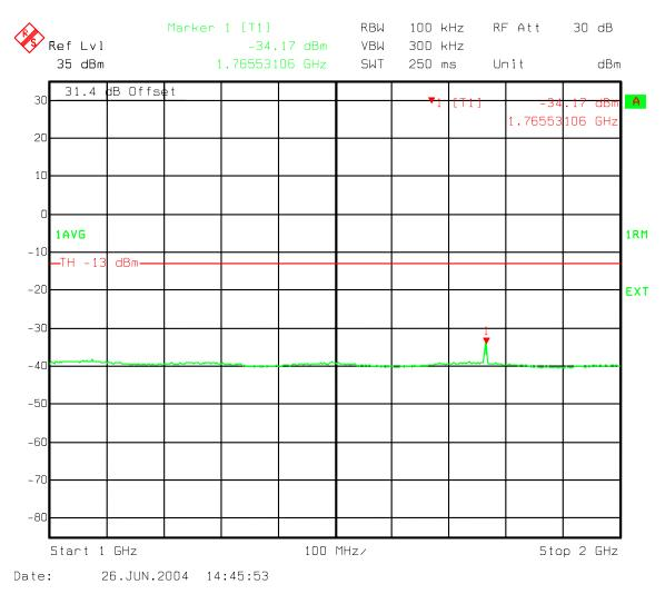
Figure 107: Three Carriers IS856 16QAM - B Band Spurious emissions 1000-2000 MHz
