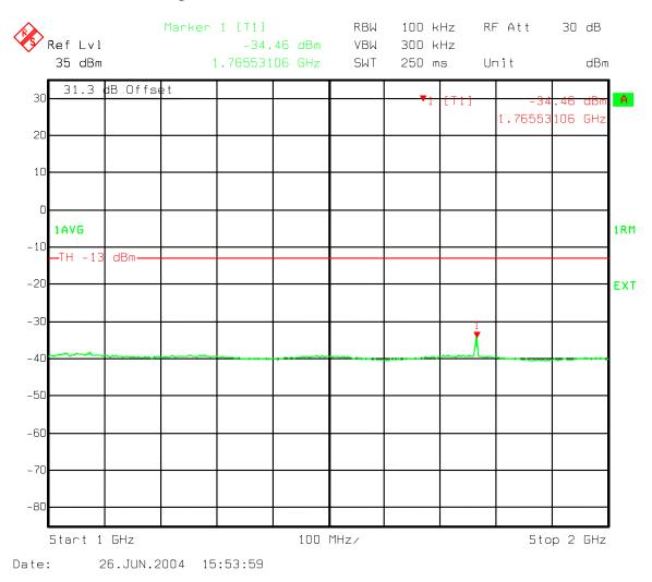
Figure 151: Three Carriers IS856 8PSK - B Band Spurious emissions 1000-2000 MHz
