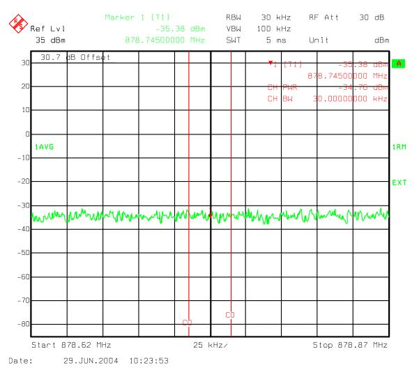
Figure 123: Combination Three Carriers 2-IS856 16QAM, 1-IS95 - Industry Canada 1.98 MHz offset Lower 30 kHz Chan Power Ch 358, 399, 440
