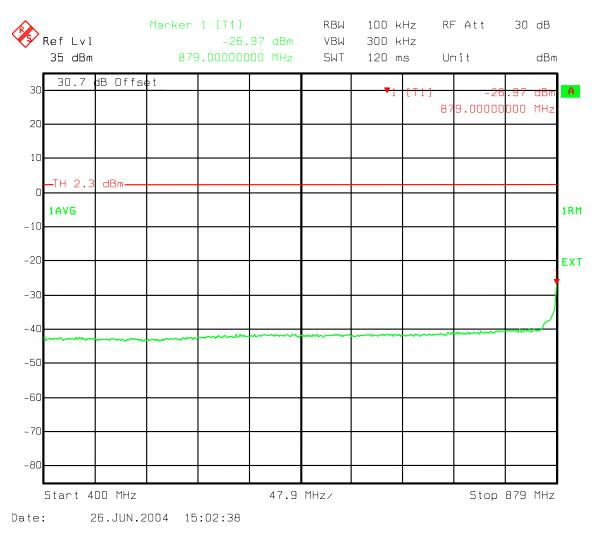
Figure 104: Three Carriers IS856 16QAM - B Band Spurious emissions 400 MHz to Lower 1 MHz Band Edge
