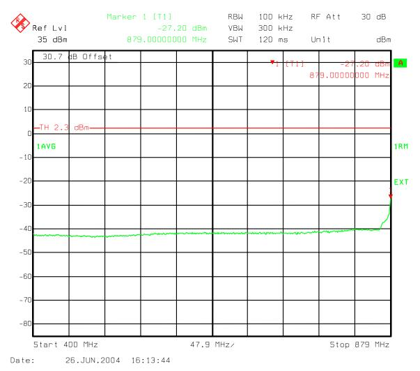
Figure 148 : Three Carriers IS856 8PSK - B Band Spurious emissions 400 MHz to Lower 1 MHz Band Edge
