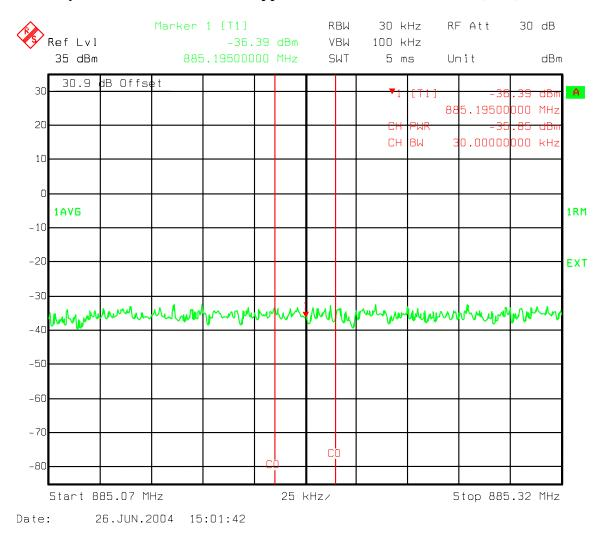
Figure 102: Three Carriers IS856 16QAM - Industry Canada 1.98 MHz offset Upper 30 kHz Chan Power Ch 358, 399, 440
