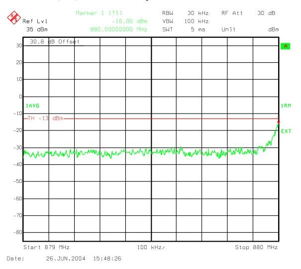
Figure 139: Three Carriers IS856 8PSK - B Band Ch 358, 399, 440 IS856 Adjacent 1MHz Lower emissions 879-880MHz
