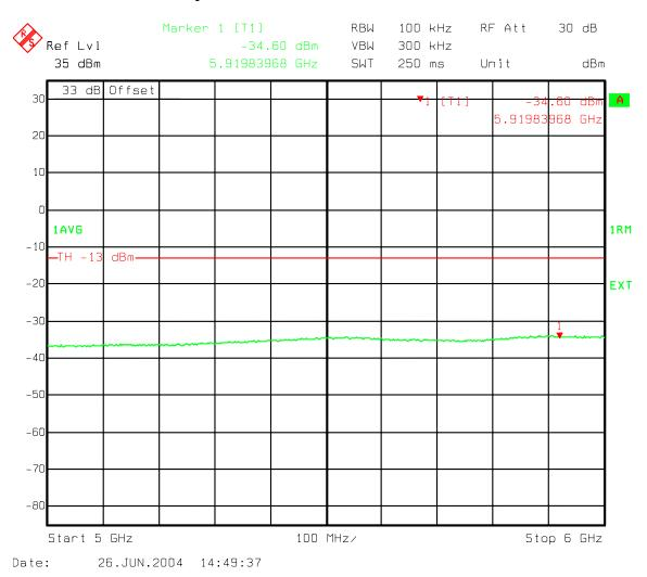
Figure 111: Three Carriers IS856 16QAM - B Band Spurious emissions 5000-6000 MHz
