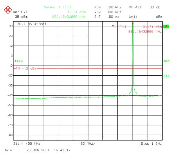
Figure 172: Three Carriers IS856 QPSK - B Band Spurious emissions 400-1000 MHz
