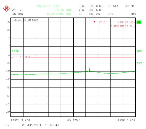
Figure 156: Three Carriers IS856 8PSK - B Band Spurious emissions 6000-7000 MHz
