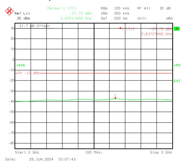
Figure 130 : Combination Three Carriers 2-IS856 16QAM, 1-IS95 - B Band Spurious emissions 2000-3000 MHz
