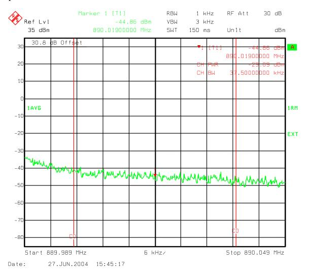
Figure 142: Three Carriers IS856 8PSK - Ch 560, 601, 642 Upper B Band adjacent to outside edge 37.5 kHz band Channel power
