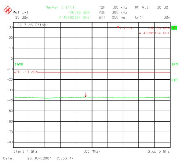
Figure 154: Three Carriers IS856 8PSK - B Band Spurious emissions 4000-5000 MHz
