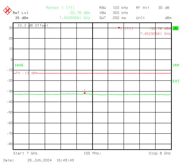
Figure 179: Three Carriers IS856 QPSK - B Band Spurious emissions 7000-8000 MHz
