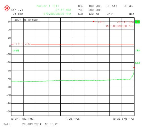
Figure 170 : Three Carriers IS856 QPSK - B Band Spurious emissions 400 MHz to Lower 1 MHz Band Edge
