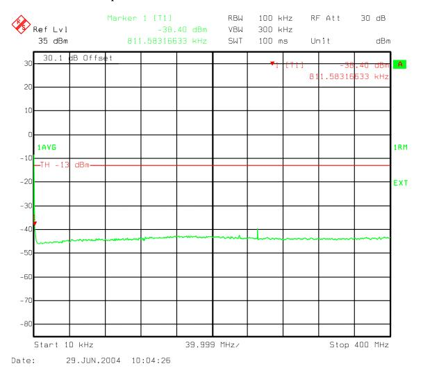
Figure 125 : Combination Three Carriers 2-IS856 16QAM, 1-IS95 - B Band Spurious emissions 10kHz-400 MHz
