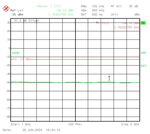
Figure 173: Three Carriers IS856 QPSK - B Band Spurious emissions 1000-2000 MHz
