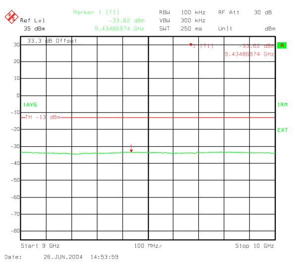
Figure 115: Three Carriers IS856 16QAM - B Band Spurious emissions 9000-10000 MHz
