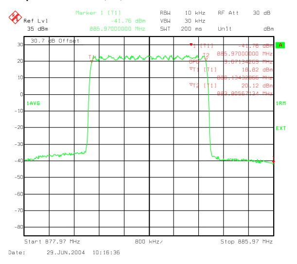
Figure 116 : Combination Three Carriers 2-IS856 16QAM, 1-IS95 - Occupied Bandwidth Ch 358, 399, 440 Band B
