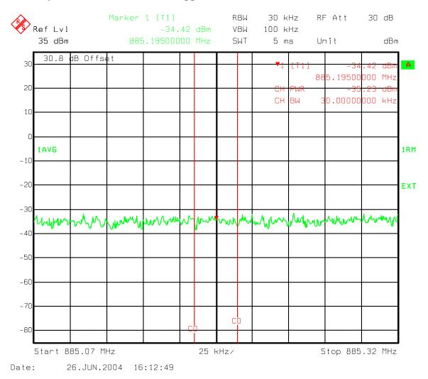
Figure 146: Three Carriers IS856 8PSK - Industry Canada 1.98 MHz offset Upper 30 kHz Chan Power Ch 358, 399, 440
