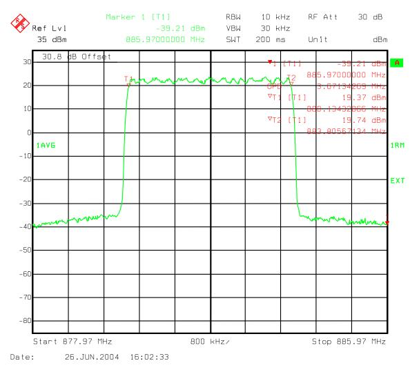
Figure 138: Three Carriers IS856 8PSK - Occupied Bandwidth Ch 358, 399, 440 Band B
