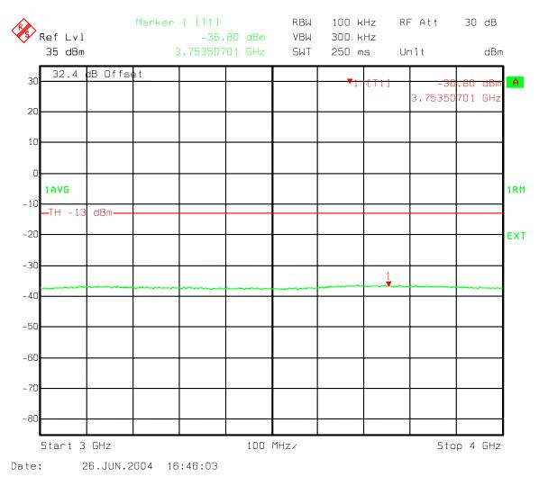
Figure 175: Three Carriers IS856 QPSK - B Band Spurious emissions 3000-4000 MHz
