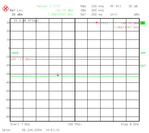
Figure 113: Three Carriers IS856 16QAM - B Band Spurious emissions 7000-8000 MHz
