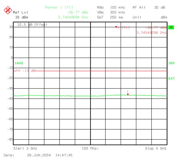
Figure 109: Three Carriers IS856 16QAM - B Band Spurious emissions 3000-4000 MHz
