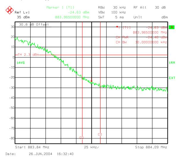
Figure 166: Three Carriers IS856 QPSK - Industry Canada Upper 750 kHz offset 30 kHz Chan Power Ch 358, 399, 440
