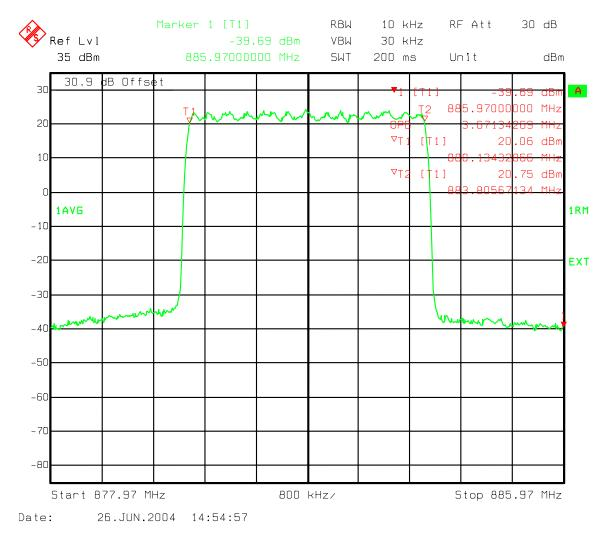
Figure 94: Three Carriers IS856 16QAM - Occupied Bandwidth Ch 358, 399, 440 Band B
