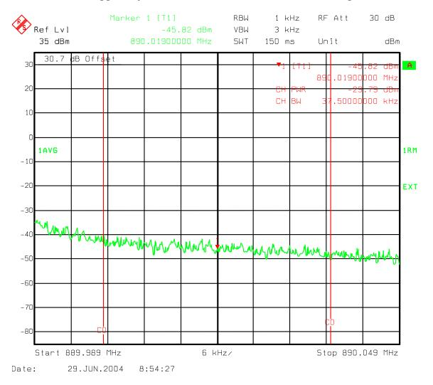
Figure 120 : Combination Three Carriers 2-IS856 16QAM, 1-IS95 - Ch 560, 601, 642 Upper B Band adjacent to outside edge 37.5 kHz band Channel power
