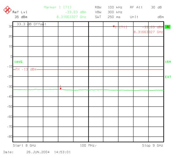
Figure 114: Three Carriers IS856 16QAM - B Band Spurious emissions 8000-9000 MHz
