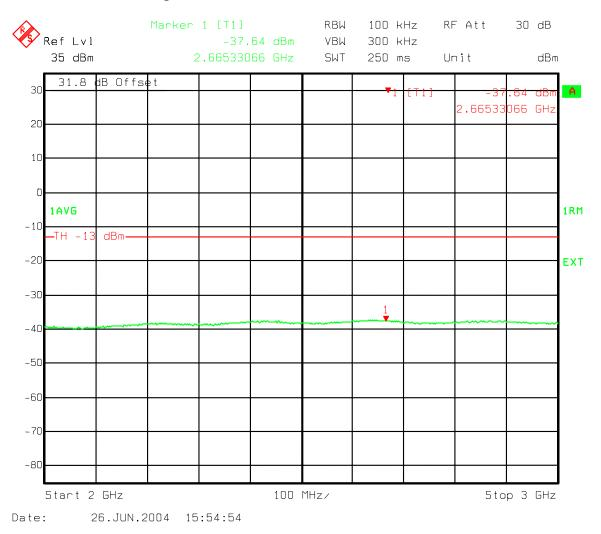
Figure 152: Three Carriers IS856 8PSK - B Band Spurious emissions 2000-3000 MHz
