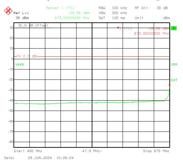
Figure 126: Combination Three Carriers 2-IS856 16QAM, 1-IS95 - B Band Spurious emissions 400 MHz to Lower 1 MHz Band Edge
