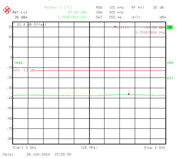
Figure 153: Three Carriers IS856 8PSK - B Band Spurious emissions 3000-4000 MHz
