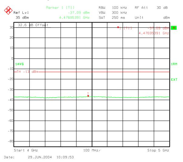
Figure 132 : Combination Three Carriers 2-IS856 16QAM, 1-IS95 - B Band Spurious emissions 4000-5000 MHz
