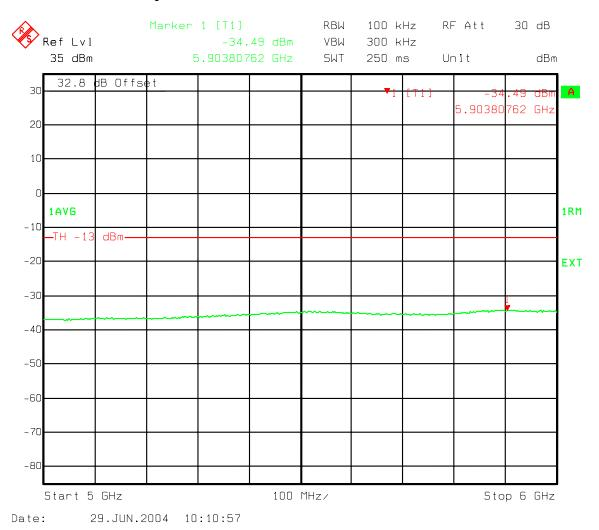
Figure 133: Combination Three Carriers 2-IS856 16QAM, 1-IS95 - B Band Spurious emissions 5000-6000 MHz
