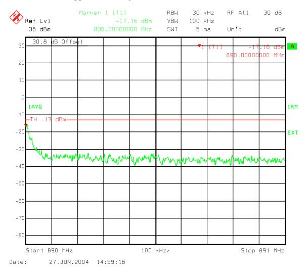
Figure 97: Three Carriers IS856 16QAM - Ch 560, 601, 642 Upper B Band adjacent 1 MHz band emissions 890-891 MHz
