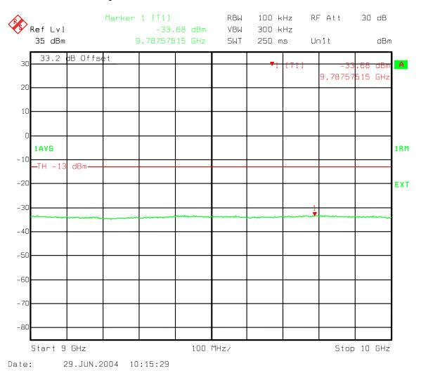
Figure 137: Combination Three Carriers 2-IS856 16QAM, 1-IS95 - B Band Spurious emissions 9000-10000 MHz
