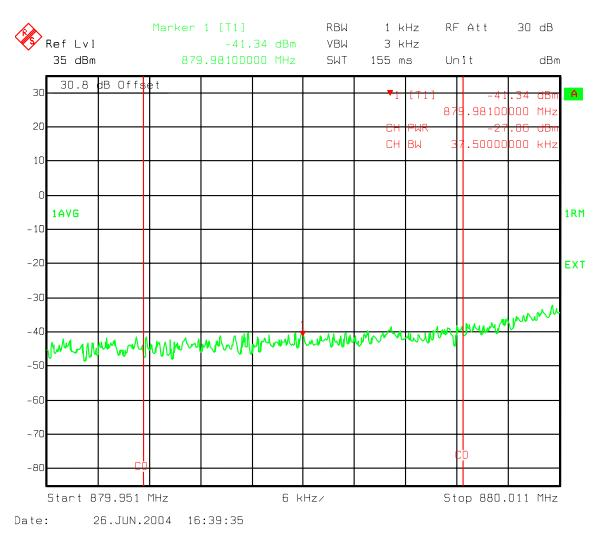
Figure 162: Three Carriers IS856 QPSK - Ch 358, 399, 440 IS856 Lower B Band Adjacent to outside edge 37.5kHz band Channel Power
