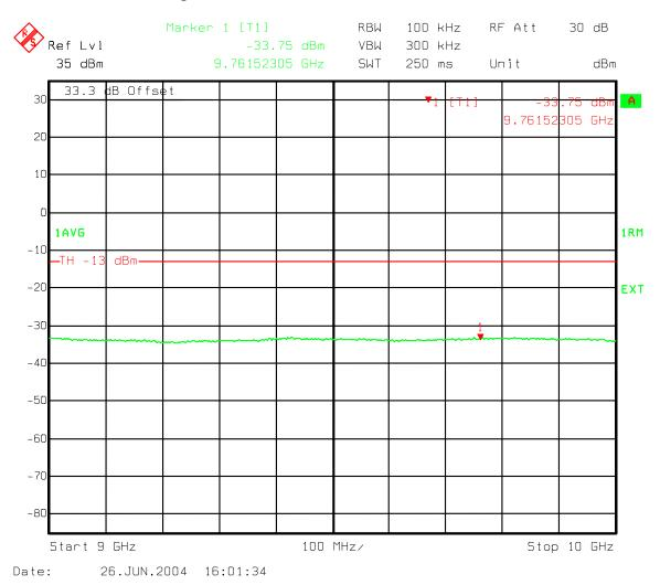
Figure 159: Three Carriers IS856 8PSK - B Band Spurious emissions 9000-10000 MHz
