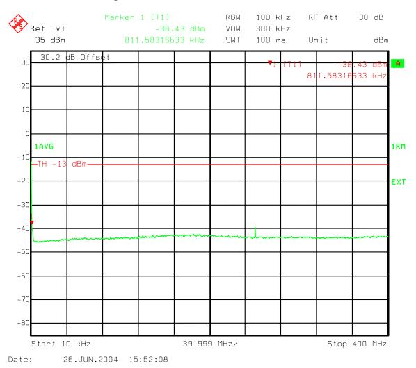
Figure 147: Three Carriers IS856 8PSK - B Band Spurious emissions 10kHz-400 MHz
