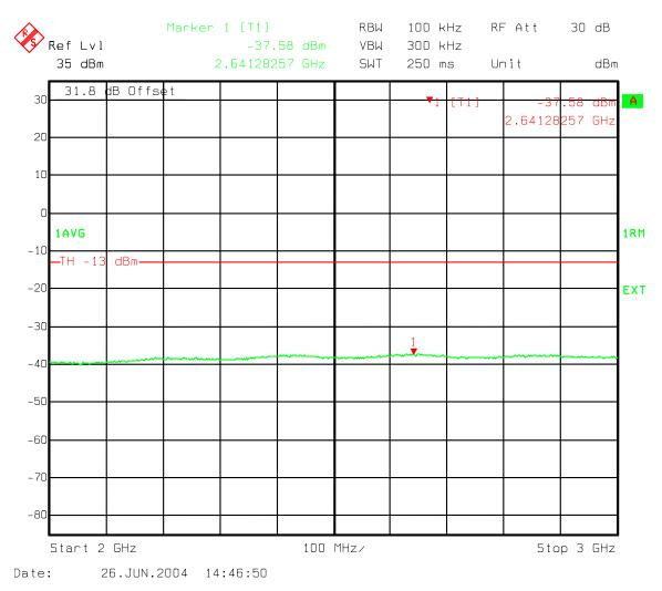
Figure 108: Three Carriers IS856 16QAM - B Band Spurious emissions 2000-3000 MHz
