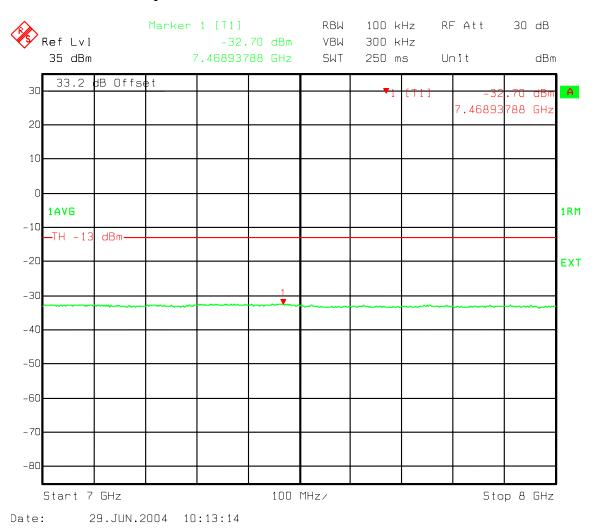
Figure 135: Combination Three Carriers 2-IS856 16QAM, 1-IS95 - B Band Spurious emissions 7000-8000 MHz
