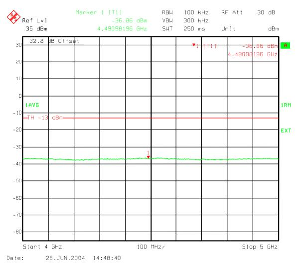
Figure 110: Three Carriers IS856 16QAM - B Band Spurious emissions 4000-5000 MHz
