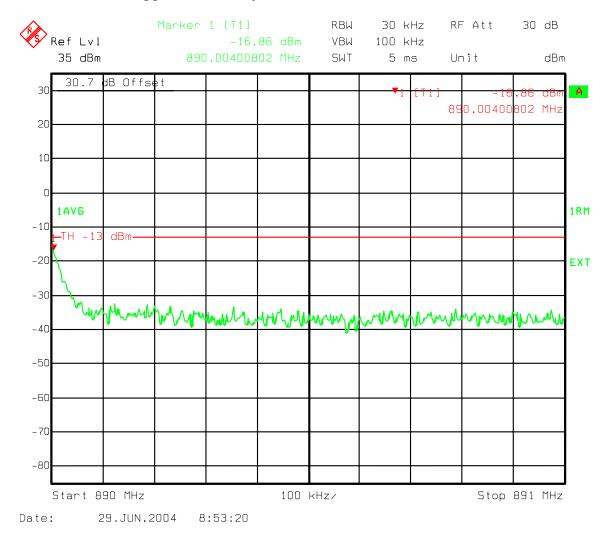
Figure 119: Combination Three Carriers 2-IS856 16QAM, 1-IS95 - Ch 560, 601, 642 Upper B Band adjacent 1 MHz band emissions 890-891 MHz
