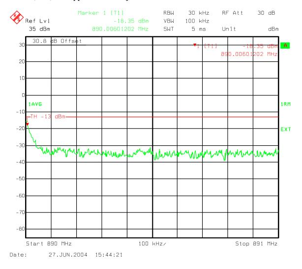
Figure 141: Three Carriers IS856 8PSK - Ch 560, 601, 642 Upper B Band adjacent 1 MHz band emissions 890-891 MHz
