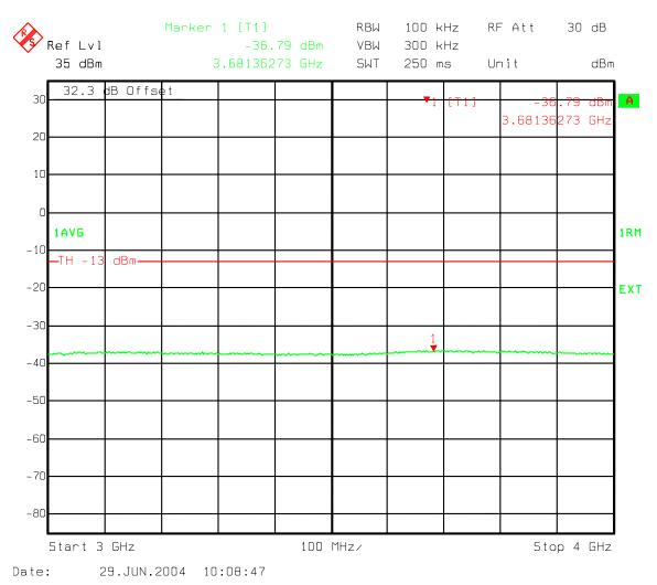
Figure 131: Combination Three Carriers 2-IS856 16QAM, 1-IS95 - B Band Spurious emissions 3000-4000 MHz
