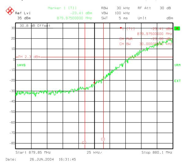
Figure 165: Three Carriers IS856 QPSK - Industry Canada Lower 750 kHz offset 30 kHz Chan Power Ch 358, 399, 440
