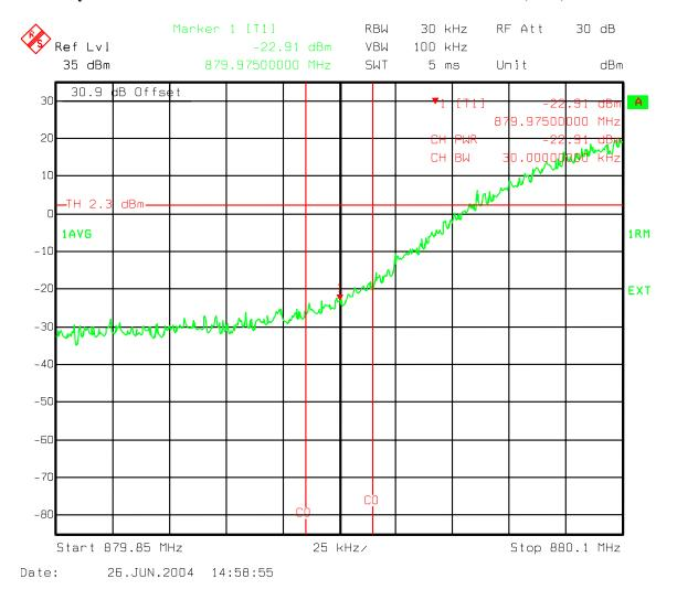
Figure 99: Three Carriers IS856 16QAM - Industry Canada Lower 750 kHz offset 30 kHz Chan Power Ch 358, 399, 440
