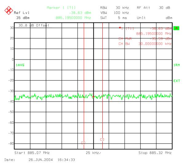
Figure 168: Three Carriers IS856 QPSK - Industry Canada 1.98 MHz offset Upper 30 kHz Chan Power Ch 358, 399, 440
