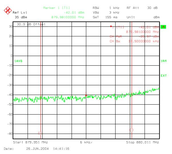
Figure 96: Three Carriers IS856 16QAM - Ch 358, 399, 440 IS856 Lower B Band Adjacent to outside edge 37.5kHz band Channel Power
