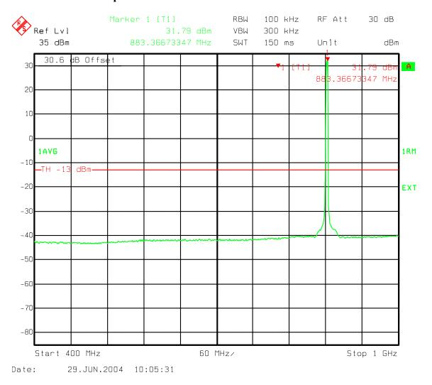
Figure 128 : Combination Three Carriers 2-IS856 16QAM, 1-IS95 - B Band Spurious emissions 400-1000 MHz
