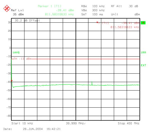
Figure 169: Three Carriers IS856 QPSK - B Band Spurious emissions 10kHz-400 MHz
