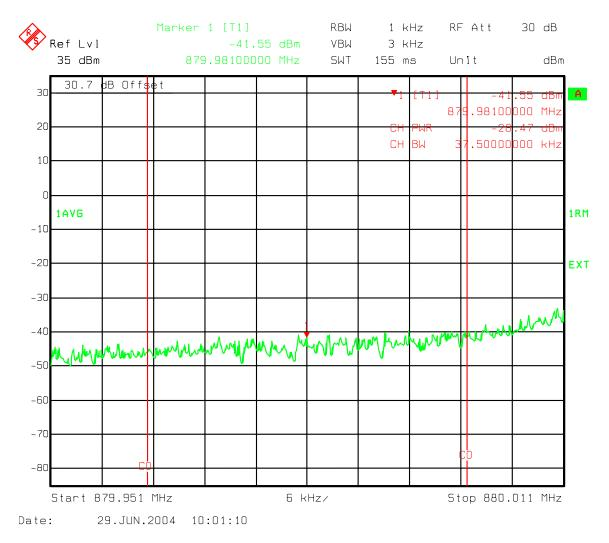
Figure 118 : Combination Three Carriers 2-IS856 16QAM, 1-IS95 - Ch 358, 399, 440 IS856 Lower B Band Adjacent to outside edge 37.5kHz band Channel Power
