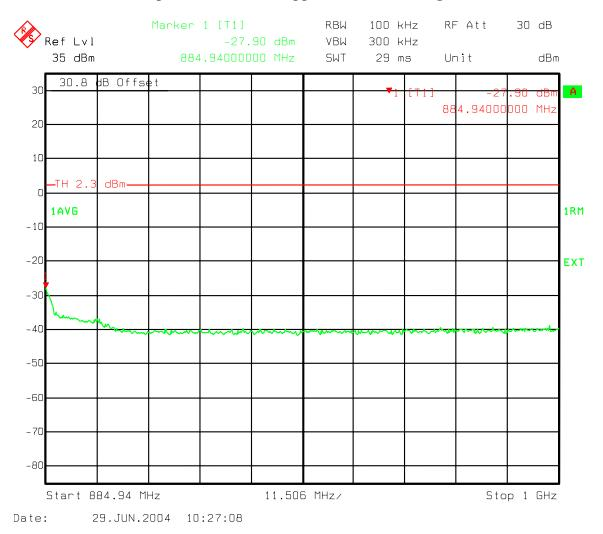
Figure 127: Combination Three Carriers 2-IS856 16QAM, 1-IS95 - B Band Spurious emissions Upper 1 MHz Band Edge to 1 GHz
