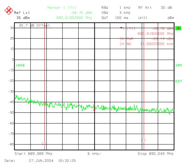
Figure 164: Three Carriers IS856 QPSK - Ch 560, 601, 642 Upper B Band adjacent to outside edge 37.5 kHz band Channel power
