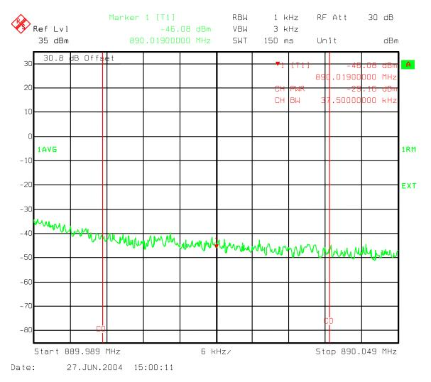
Figure 98: Three Carriers IS856 16QAM - Ch 560, 601, 642 Upper B Band adjacent to outside edge 37.5 kHz band Channel power
