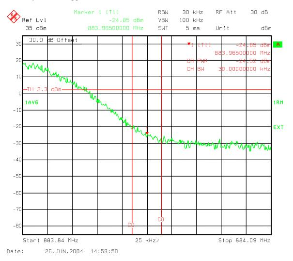
Figure 100 : Three Carriers IS856 16QAM - Industry Canada Upper 750 kHz offset 30 kHz Chan Power Ch 358, 399, 440
