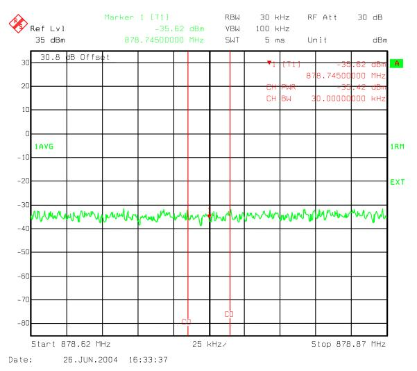
Figure 167: Three Carriers IS856 QPSK - Industry Canada 1.98 MHz offset Lower 30 kHz Chan Power Ch 358, 399, 440
