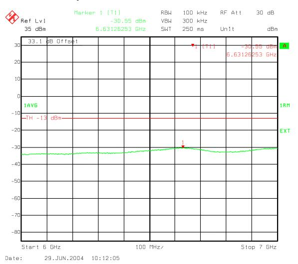
Figure 134 : Combination Three Carriers 2-IS856 16QAM, 1-IS95 - B Band Spurious emissions 6000-7000 MHz
