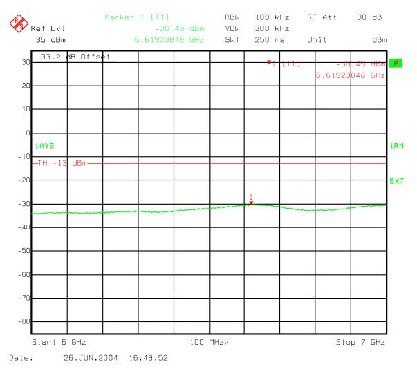
Figure 178: Three Carriers IS856 QPSK - B Band Spurious emissions 6000-7000 MHz
