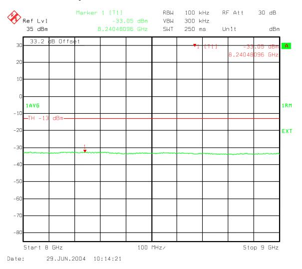
Figure 136 : Combination Three Carriers 2-IS856 16QAM, 1-IS95 - B Band Spurious emissions 8000-9000 MHz
