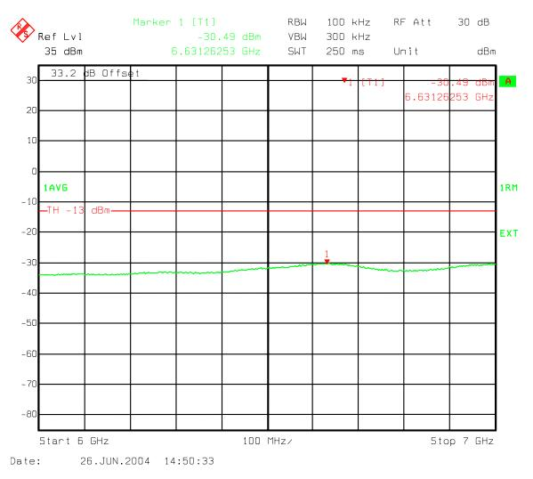
Figure 112: Three Carriers IS856 16QAM - B Band Spurious emissions 6000-7000 MHz
