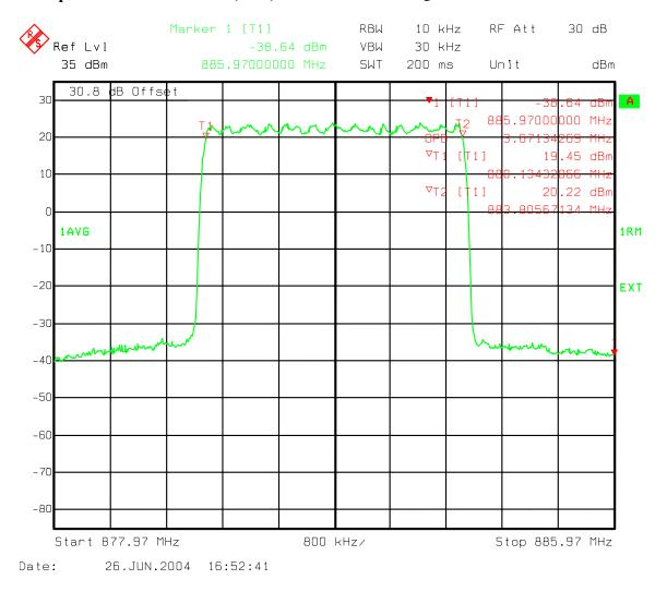
Figure 160: Three Carriers IS856 QPSK - Occupied Bandwidth Ch 358, 399, 440 Band B
