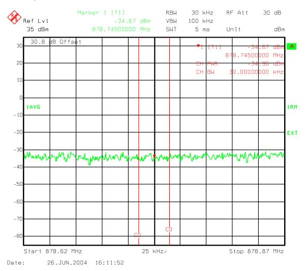
Figure 145: Three Carriers IS856 8PSK - Industry Canada 1.98 MHz offset Lower 30 kHz Chan Power Ch 358, 399, 440
