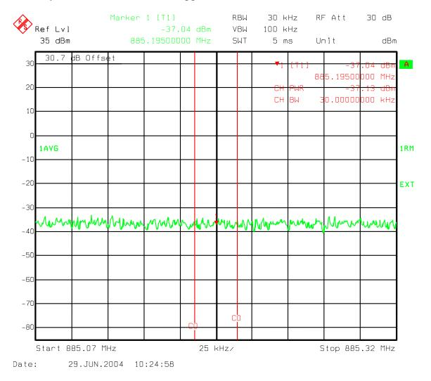
Figure 124 : Combination Three Carriers 2-IS856 16QAM, 1-IS95 - Industry Canada 1.98 MHz offset Upper 30 kHz Chan Power Ch 358, 399, 440
