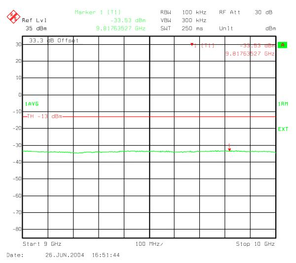
Figure 181: Three Carriers IS856 QPSK - B Band Spurious emissions 9000-10000 MHz
