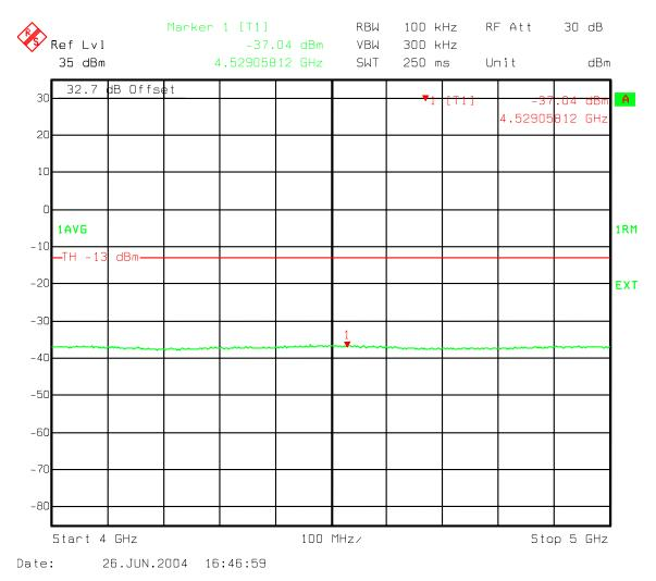
Figure 176: Three Carriers IS856 QPSK - B Band Spurious emissions 4000-5000 MHz
