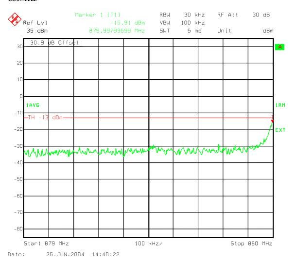
Figure 95: Three Carriers IS856 16QAM - B Band Ch 358, 399, 440 IS856 Adjacent 1MHz Lower emissions 879-880MHz
