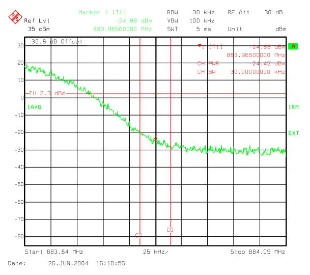
Figure 144: Three Carriers IS856 8PSK - Industry Canada Upper 750 kHz offset 30 kHz Chan Power Ch 358, 399, 440
