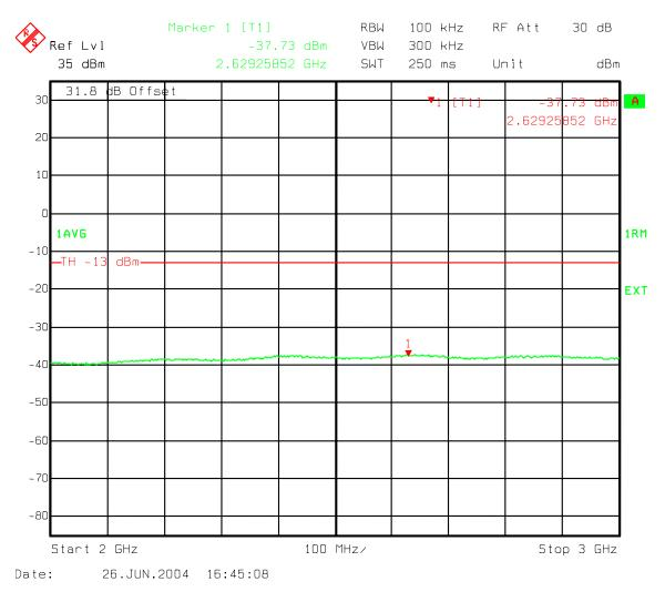
Figure 174: Three Carriers IS856 QPSK - B Band Spurious emissions 2000-3000 MHz
