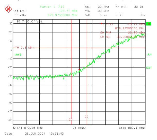
Figure 121: Combination Three Carriers 2-IS856 16QAM, 1-IS95 - Industry Canada Lower 750 kHz offset 30 kHz Chan Power Ch 358, 399, 440
