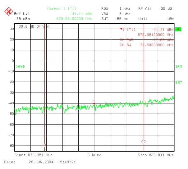
Figure 140 : Three Carriers IS856 8PSK - Ch 358, 399, 440 IS856 Lower B Band Adjacent to outside edge 37.5kHz band Channel Power
