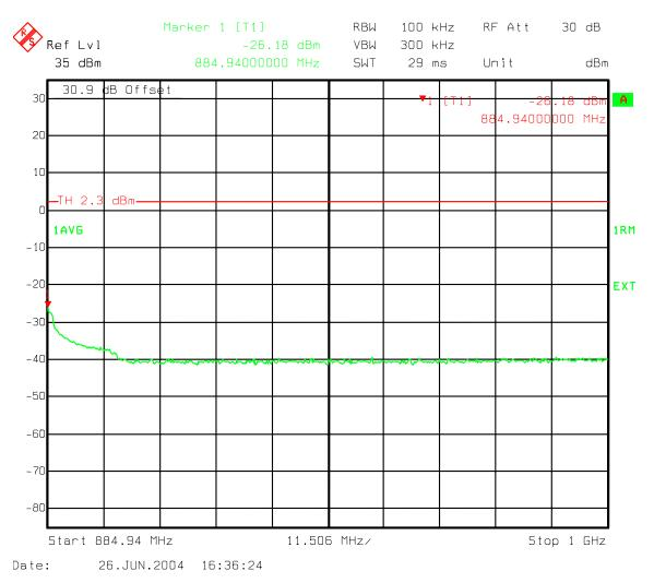
Figure 171: Three Carriers IS856 QPSK - B Band Spurious emissions Upper 1 MHz Band Edge to 1 GHz
