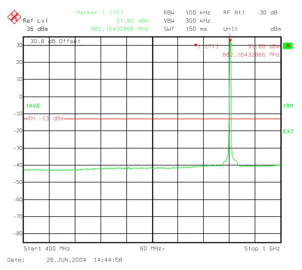
Figure 106: Three Carriers IS856 16QAM - B Band Spurious emissions 400-1000 MHz
