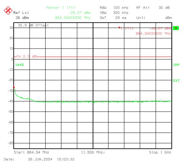
Figure 105 : Three Carriers IS856 16QAM - B Band Spurious emissions Upper 1 MHz Band Edge to 1 GHz
