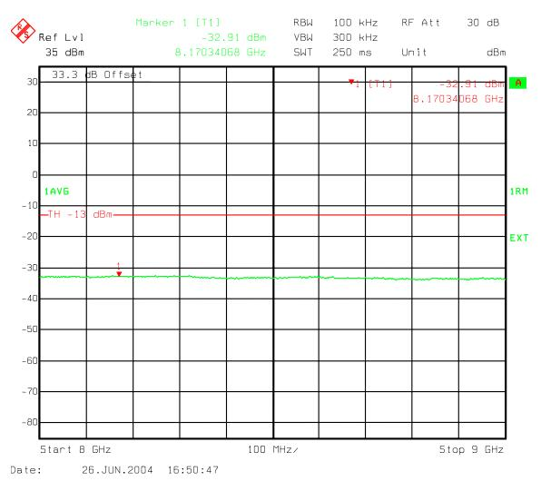
Figure 180: Three Carriers IS856 QPSK - B Band Spurious emissions 8000-9000 MHz
