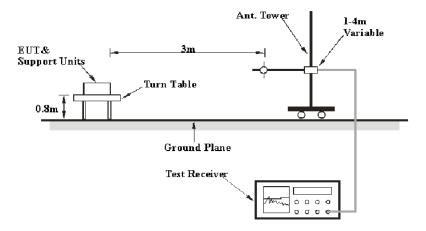
The radiated emission below 960MHz tests were performed in the 3 meters chamber test site A, using the setup accordance with the ANSI C63.10-2013. The specification used was the FCC 15.209, and FCC 15.250 limits.
