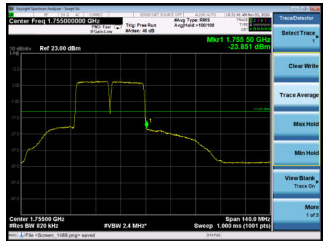
CA-4C-12A 16QAM 20MHz+20MHz+20MHz CH-High, 1 RB
