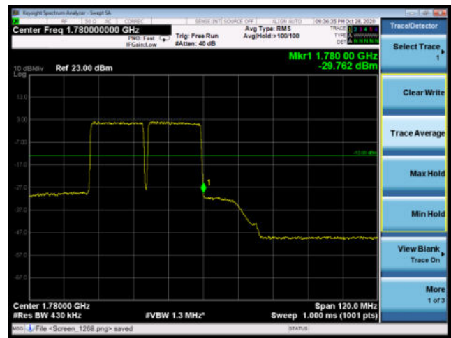
CA_66C 64QAM 20MHz+20MHz CH-High, 1 RB
