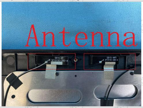
The antenna is integrated on the main PCB and no consideration of replacement. The best case gain of the antenna is1.99 dBi
