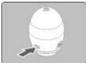
Press and hold the power button for 2 seconds.
