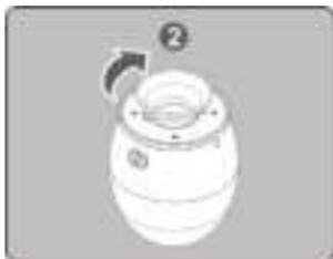
Fasten the adaptor by turning it gently in the clockwise direction.
