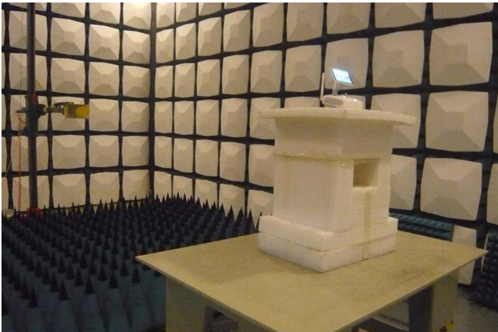
Radiated Emission Above 1GHz View
