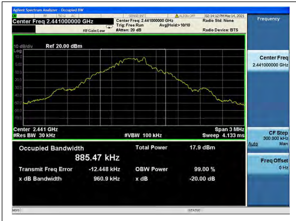
(GFSK, Channel 39, 2441MHz)
