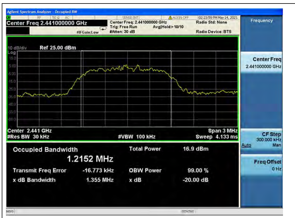
( \pi/4 -DQPSK, Channel 39, 2441MHz)
