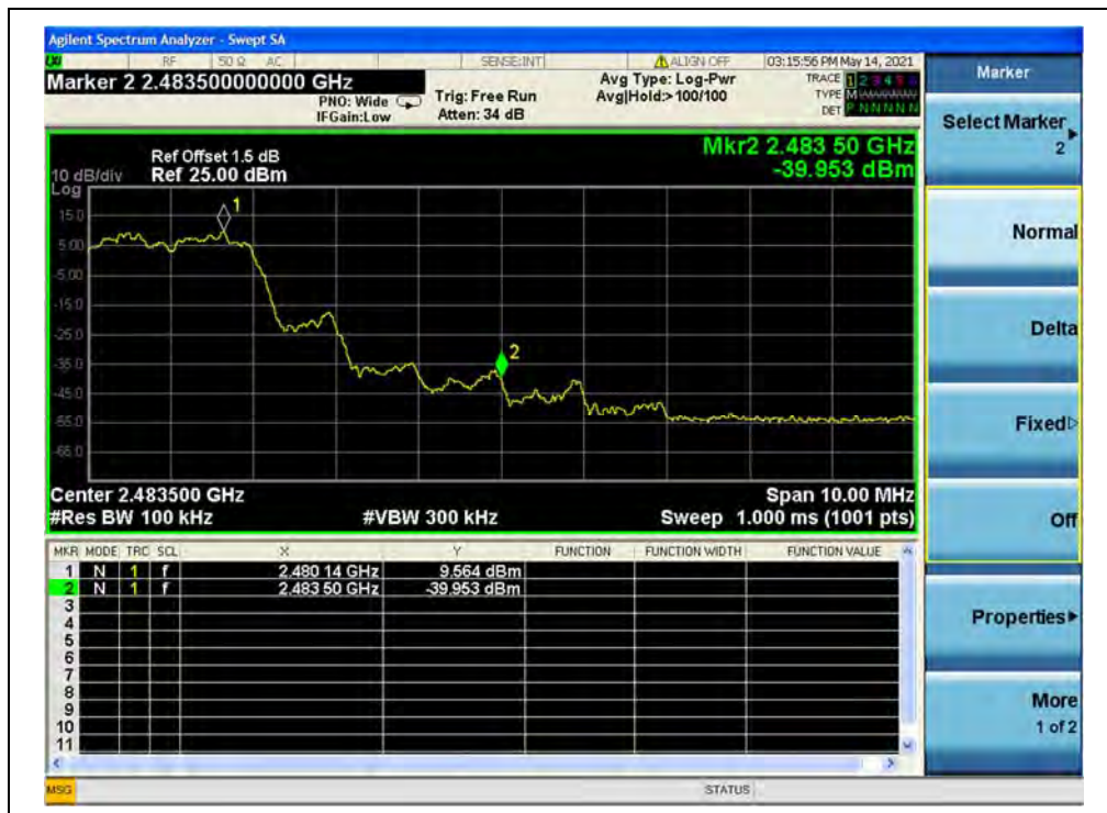
(Channel = 78, Band edge with hopping on, 8-DPSK)
