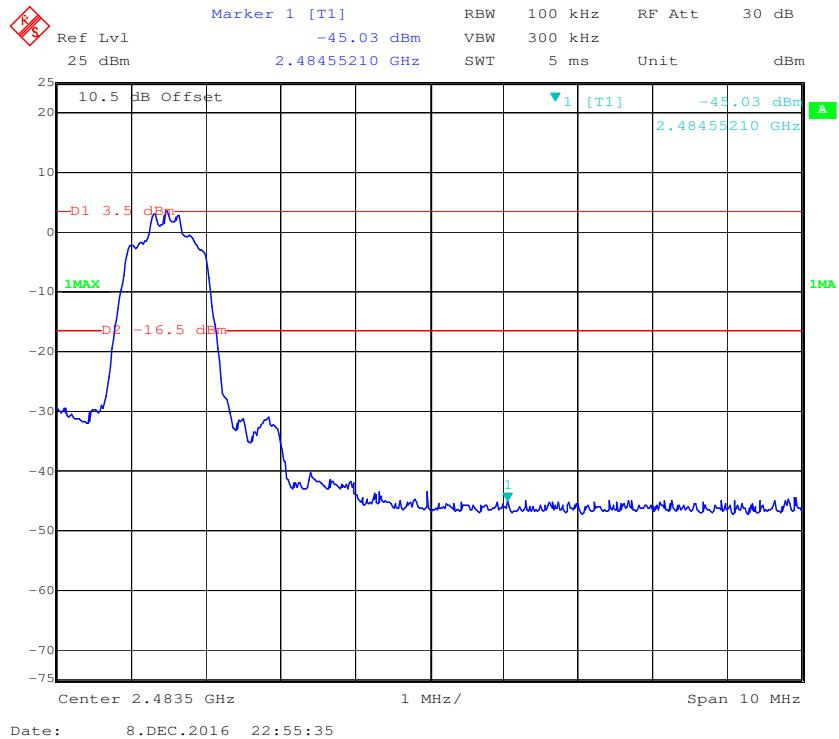
**EDR (8DPSK): Band Edge-Left Side**
