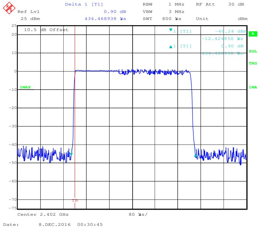
**Pulse time, Middle Channel, 2DH1**
