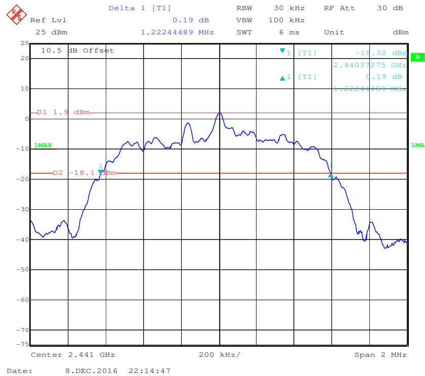
**EDR ( $\pi/4$ -DQPSK): High Channel**
