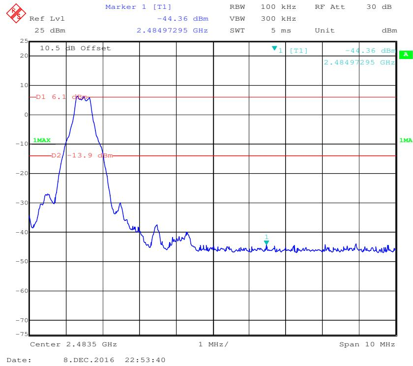
**EDR ( $\pi/4$ -DQPSK): Band Edge-Left Side**
