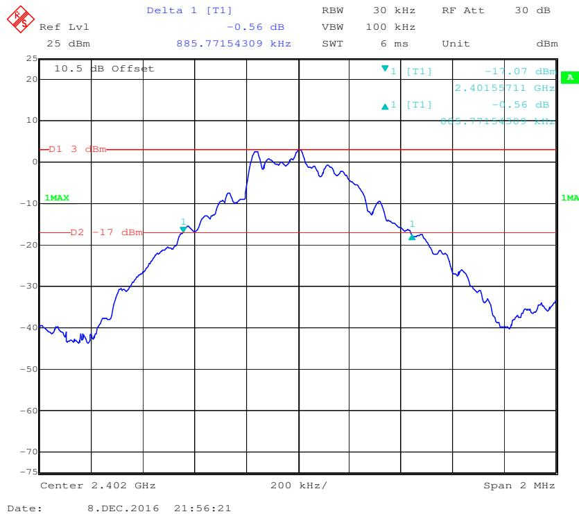
**BDR (GFSK): Middle Channel**
