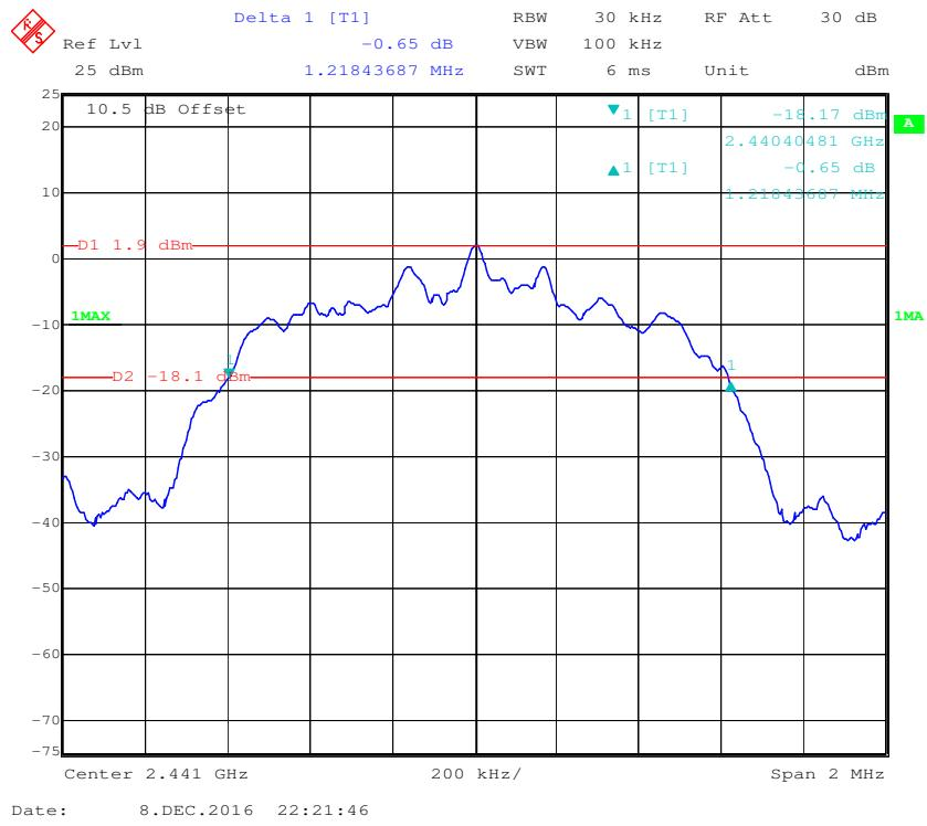
**EDR (8DPSK): High Channel**
