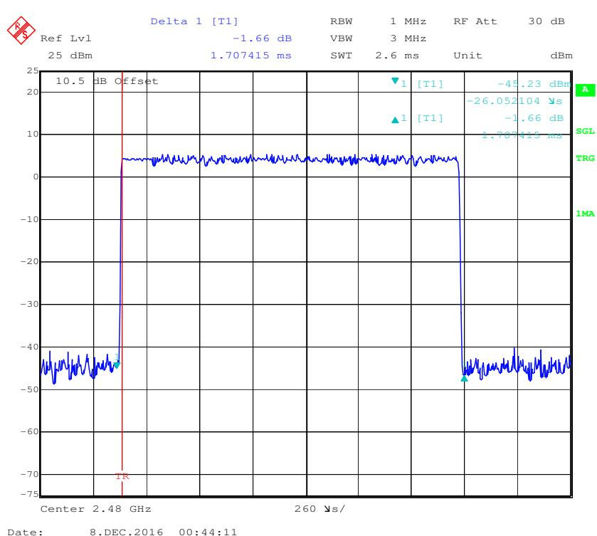
**Pulse time, Low Channel, 3DH5**
