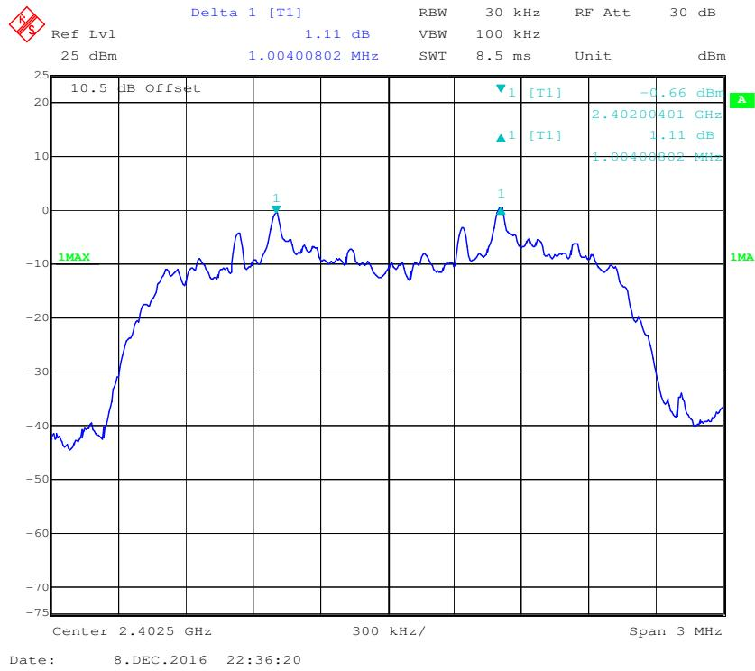
**EDR ( $\pi/4$ -DQPSK): Middle Channel**
