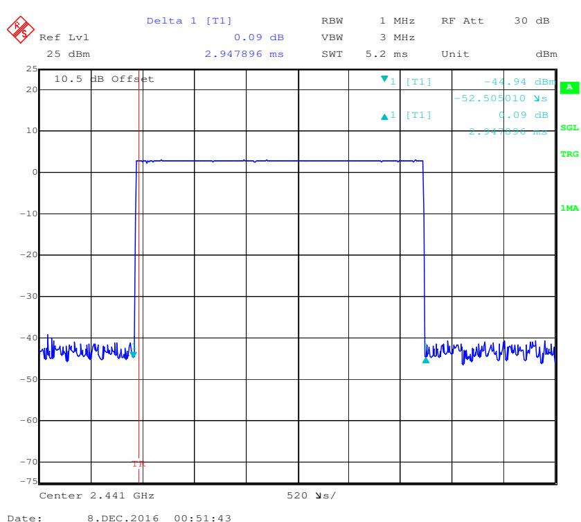
**Pulse time, High Channel, DH5**
