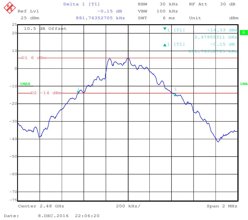
**EDR ( $\pi/4$ -DQPSK): Low Channel**
