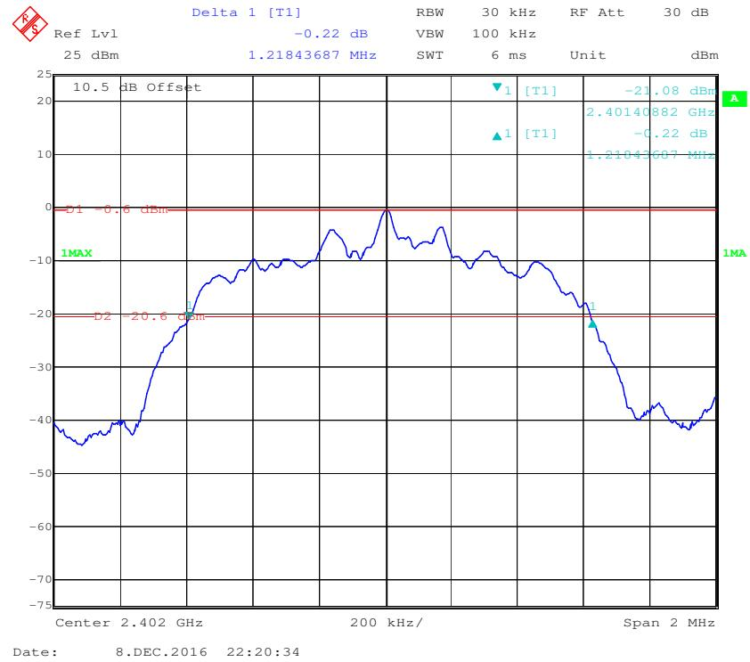
**EDR (8DPSK): Middle Channel**
