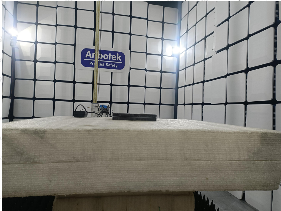
Photo of Radiation Emission Test (above 1GHz)
