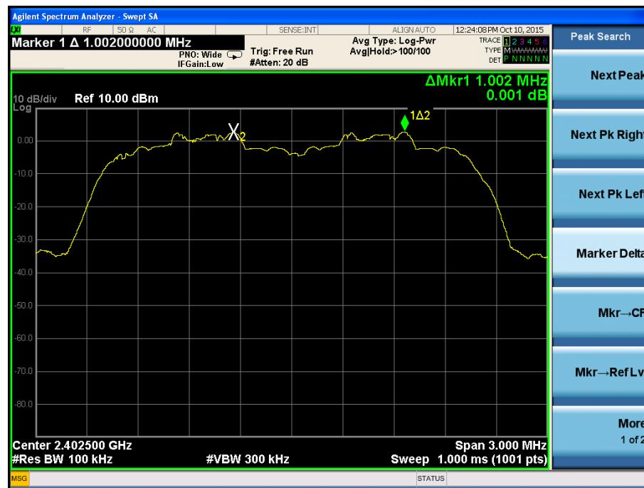
Channel Spacing (Middle CH=1MHz)
