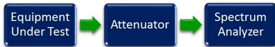
Figure 1 Output RF power Test Setup
