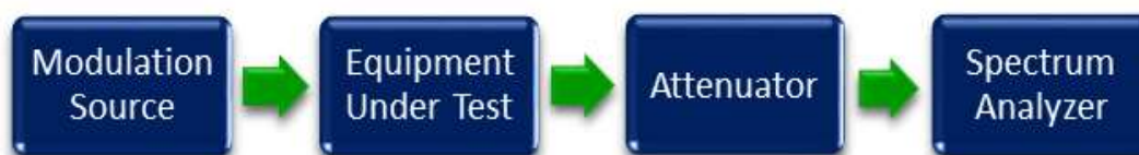
Figure 2: Occupied Bandwidth Test Setup
