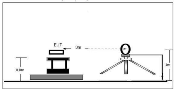
(B) Radiated Emission Test-Up Frequency 30MHz~1GHz
