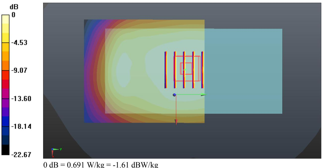
**22\_LTE Ban66\_20M\_QPSK\_100RB\_0Offset\_Back\_10mm\_Hotspot On\_Ch132572**
