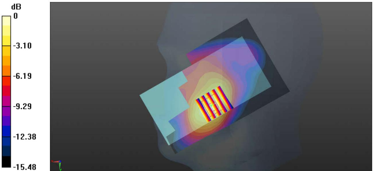
**10\_LTE Band2\_20M\_QPSK\_1RB\_49Offset\_Right Cheek\_0mm\_Ch18900**
