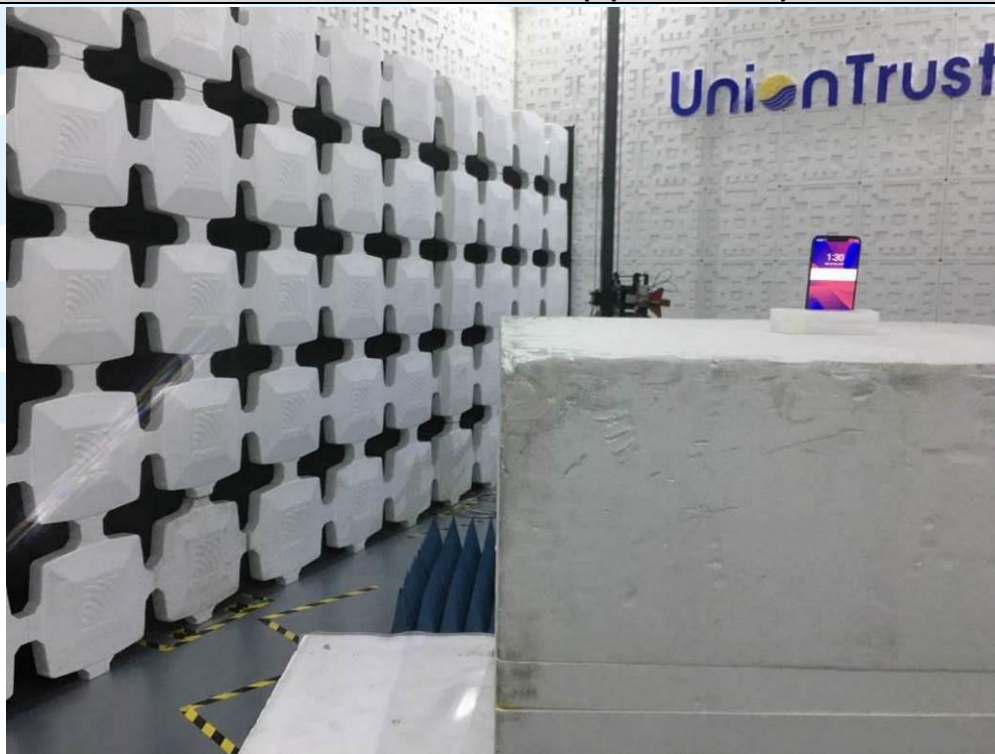
Radiated emission Test Setup (Above 1 GHz)
