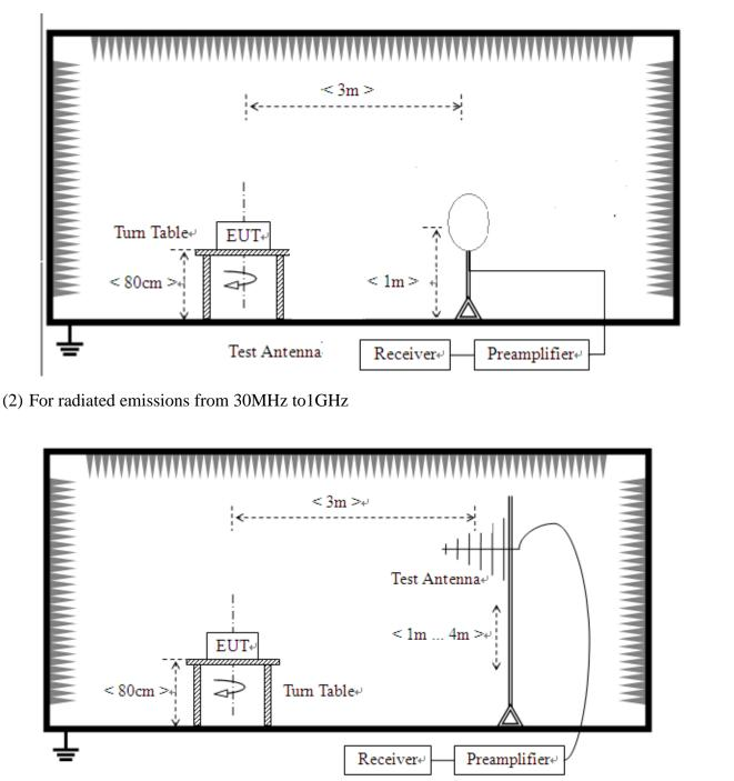
The test site semi-anechoic chamber has met the requirement of NSA tolerance 4 dB according to the standards: ANSI C63.10:2013. The EUT was set-up on insulator 80cm above the Ground Plane. The set-up and test methods were according to ANSI C63.10:2013.
