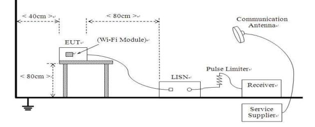
The Table-top EUT was placed upon a non-metallic table 0.8m above the horizontal metal reference ground plane. EUT was connected to LISN and LISN was connected to reference Ground Plane. EUT was 80cm from LISN. The set-up and test methods were according to ANSI C63.10:2013:2009
