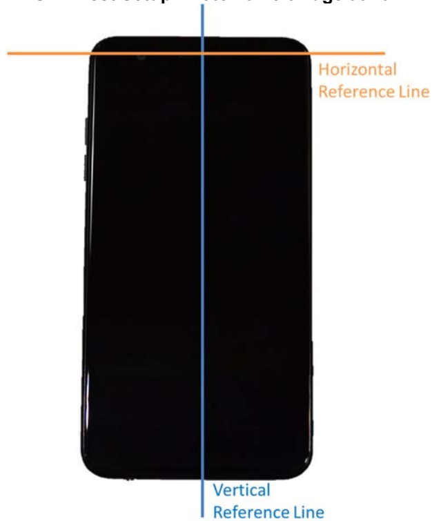
SAR Test Setup Photo 11 Horizontal and Vertical Reference Lines
